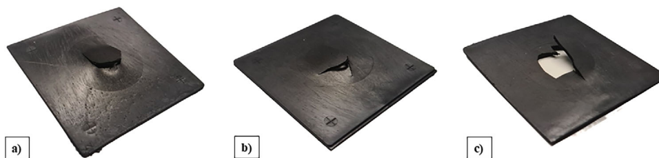
FIGURE 8 | Specimens after falling weight tests (a) TDV_MFI2, (b) TDV_MFI12, (c) TDV_MFI45.
