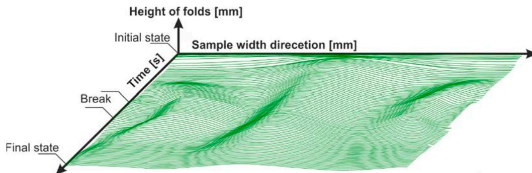
**Figure 6.** Measured height profile of the laser beam as a function of time (SDK software, Basler) over a constant width of 150 mm—carbon fiber (CF) biaxial non-crimp fabric  $\pm 45^\circ$ , ST  $0^\circ$ ; Hysteresis with 10 seconds break at maximum deflection.
