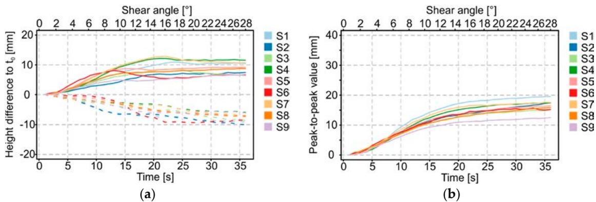
**Figure 17.** Amplitudes of maxima and minima (a). Peak-to-peak value (b). CF biaxial non-crimp fabric  $\pm 45^\circ$ , ST  $0^\circ$ , nine samples.
