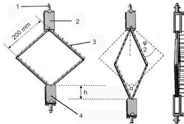
**Figure 3.** Modified picture frame (1: adapter; 2: upper frame holder; 3: needle bar; 4: lower frame holder).
