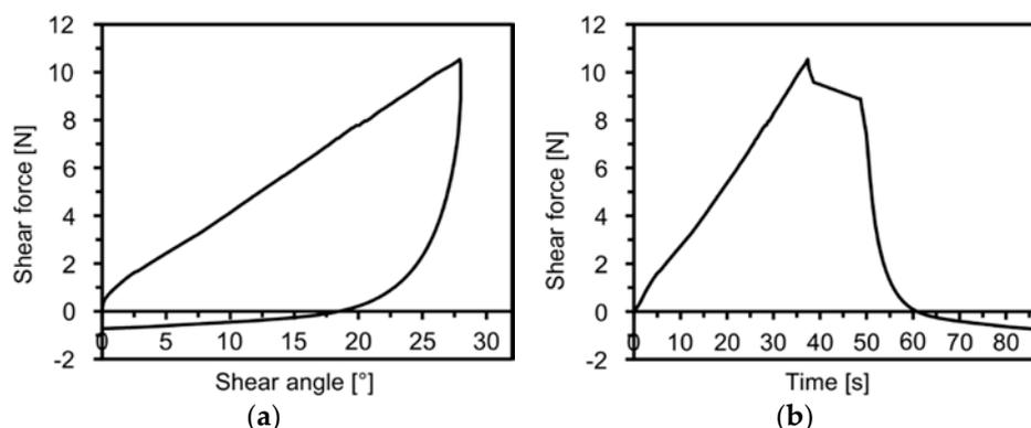
**Figure 7.** Shear force/shear angle diagram (a). Shear force/time diagram (b) for a CF-biaxial non-crimp fabric.
