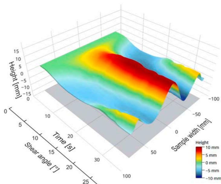
**Figure 16.** Deflection of the laser beam over time of CF biaxial non-crimp fabric  $\pm 45^\circ$ , ST  $0^\circ$ .
