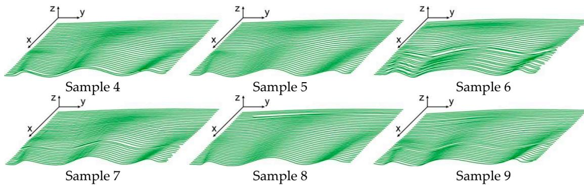
**Figure 15.** Measured height profiles of the laser beam as a function of time—CF biaxial non-crimp fabric  $\pm 45^\circ$ , ST  $0^\circ$ ; x-axis: time; y-axis: width; z-axis: height (also see Figure 6)
