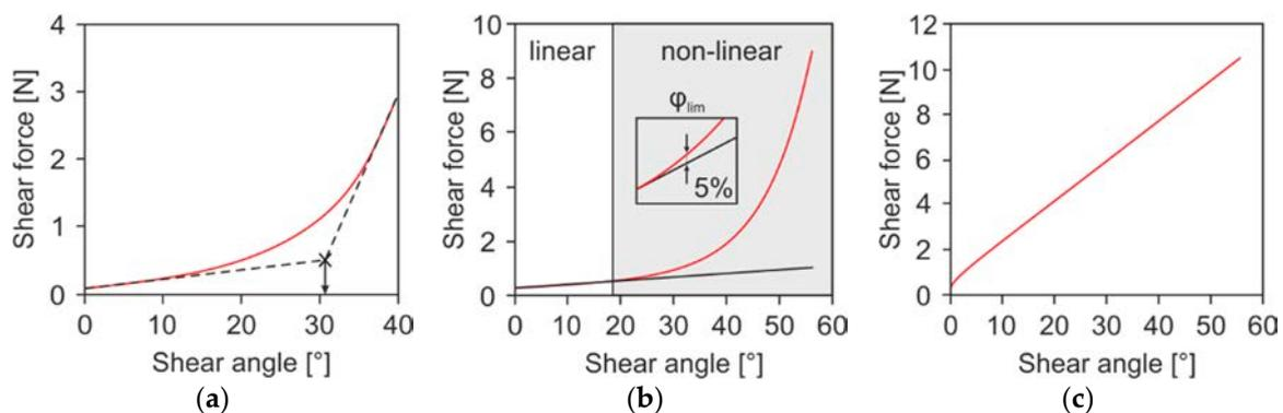
**Figure 2.** Evaluation of a shear force/shear angle diagram. Determination of the critical shear angle (a) according to [37] and (b), according to [38,39], (c) shear force/shear angle diagram, biaxial non-crimp fabric  $\pm 45^\circ$ , sewing thread (ST)  $0^\circ$ .
