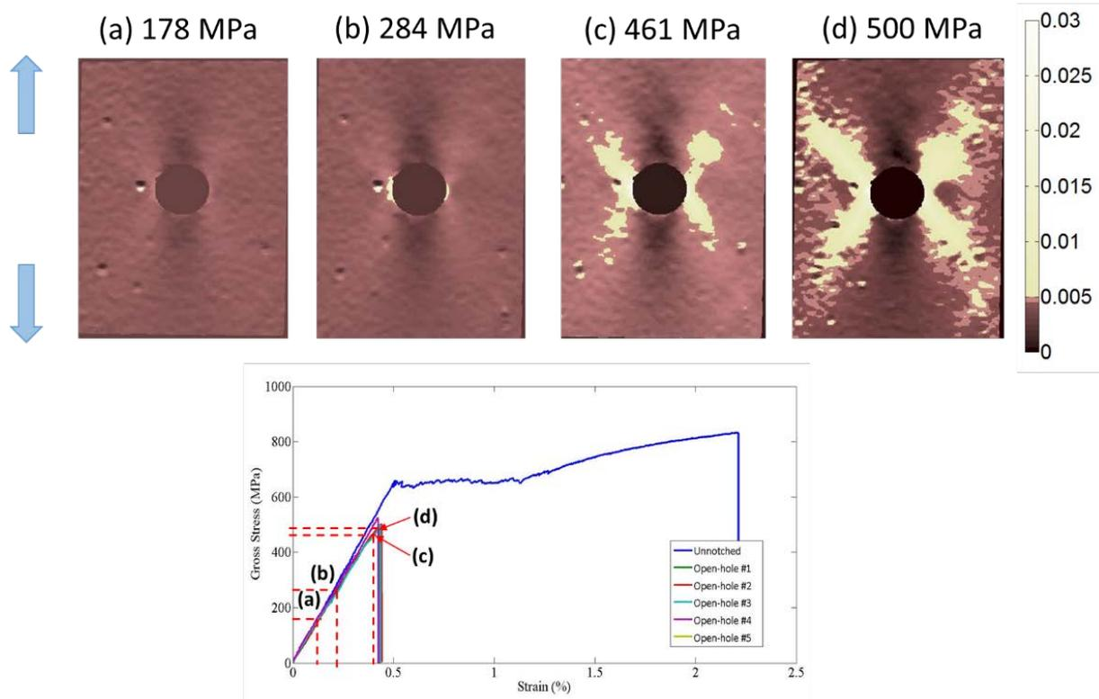
**Figure 7.** Spread of fragmentation in  $[\pm 25_2/0]_{s4}$  IM-HM carbon/epoxy laminates [8].
