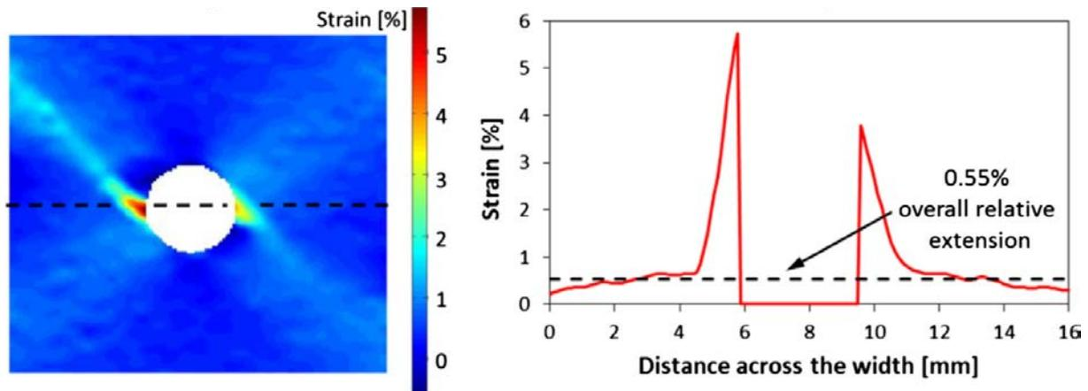
**Figure 6.** Strains in the loading direction (vertical) on carbon/carbon hybrids [6].
