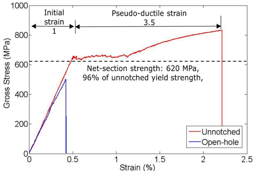
**Figure 4.** Open-hole response of  $[\pm 25_2/0]_{s4}$  IM-HM carbon/epoxy laminates.
