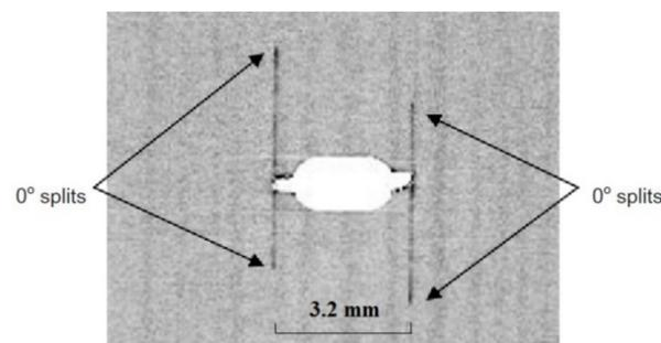
**Figure 5.** Typical splits at the centre of a  $[45/90/-45/0]_{4s}$  IM7/8552 carbon/epoxy laminate [9].
