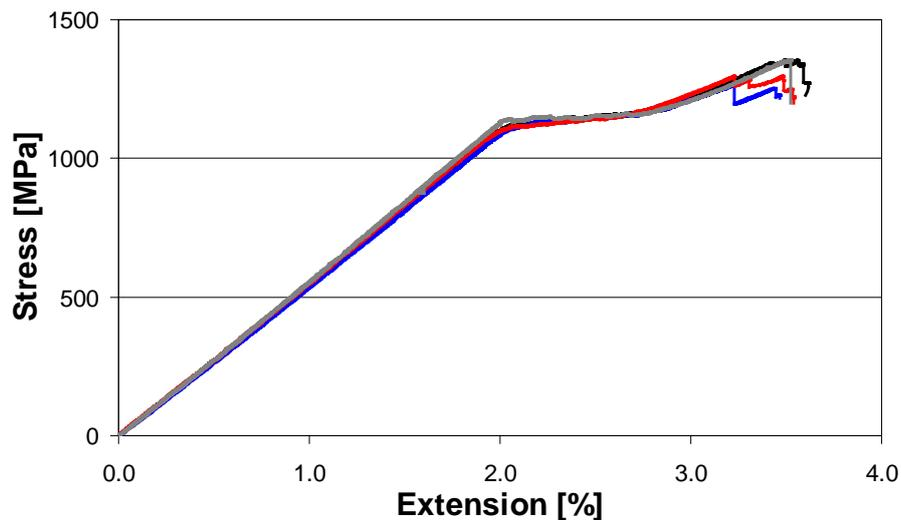
**Figure 1.** Pseudo-ductile response of S-glass/high strength carbon hybrid [1].
