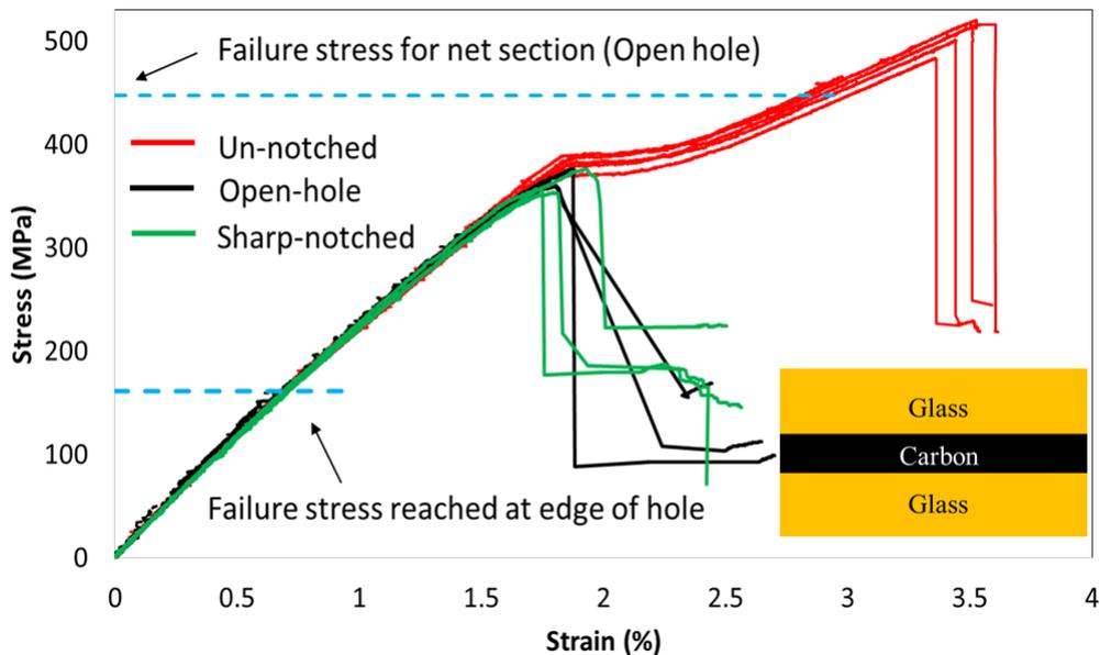
**Figure 3.** Open hole, sharp notched and unnotched response of QI  $\pm 60/0$  glass/carbon laminates [7].
