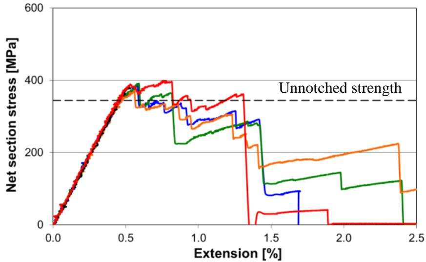
**Figure 2.** Open-hole tension of QI hybrid carbon specimens.
