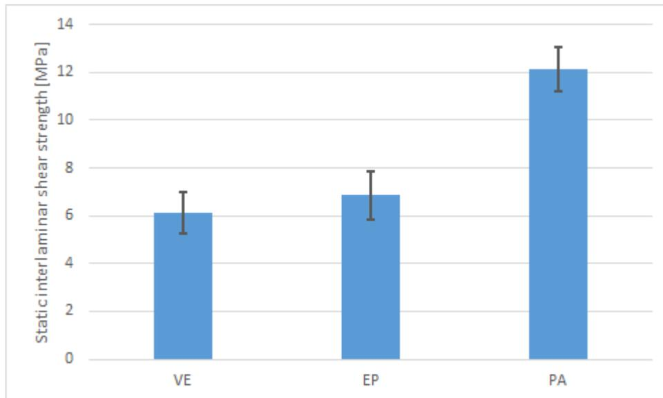
**Figure 2.** Results of the static interlaminar shear tests
