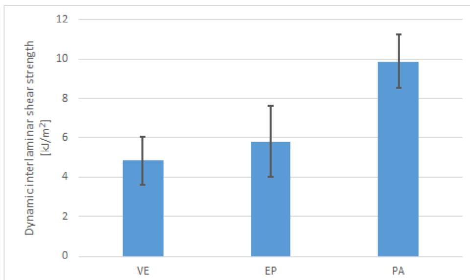
**Figure 3.** Results of the dynamic interlaminar shear tests
