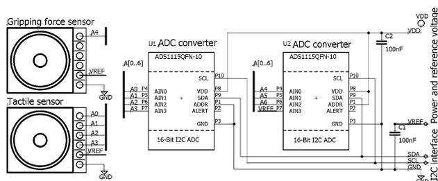
**Fig. 6** Architecture of the PCB to be integrated into the laparoscope head. The hybrid circuit contains two AD converters and two force sensors
