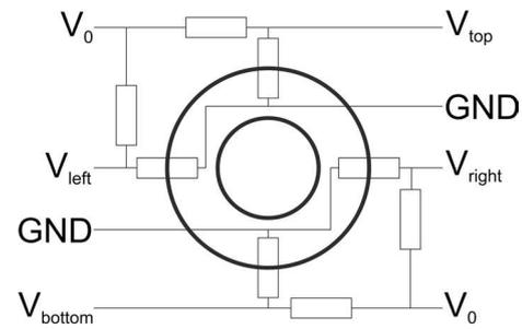
**Fig. 2** Structure and read-out of the four half Wheatstone-bridges, each formed by an active piezoresistor and one identical reference element
