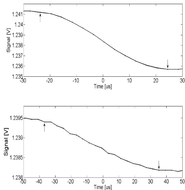
**Fig. 10** Response time of the bare (*top*) and PDMS coated (*bottom*) force sensors for perpendicular load. The arrows indicate the excitation and the signal saturation. The measured value must be reduced by  $11.8 \mu\text{s}$  delay of the actuator piezo crystal
