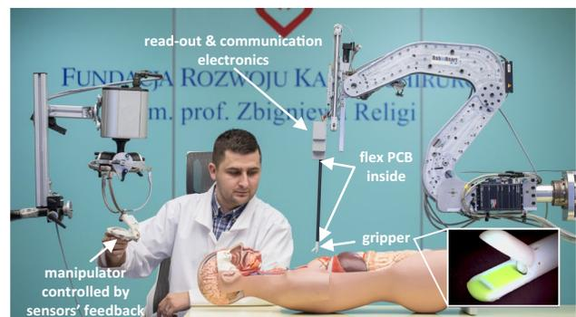
**Fig. 11** The laparoscope integrated in the Robin Heart surgery tool. The inset shows the completed grasping head
