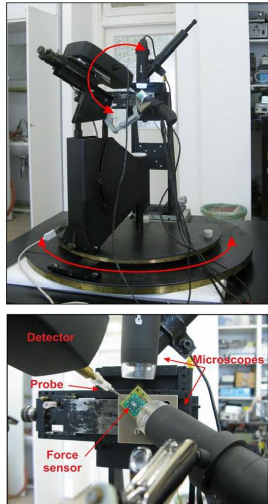
**Fig. 5** Measuring setup (top) for characterization of the sensor chips exposed to any load direction from a 1/4 of the semi-sphere. Close view of the probe head with a PCB mounted force sensor (bottom). Two cameras facilitate precise positioning
