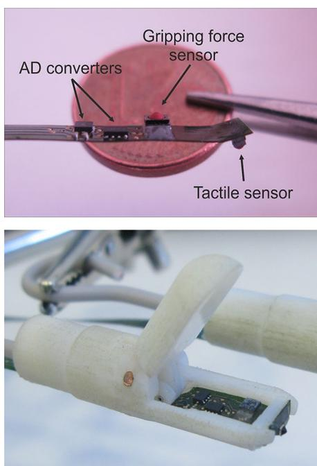
**Fig. 7** Sensor chips and AD converters integrated on the head of the 35 cm long flexible PCB. This end of the PCB is inserted in the grasper. Note that the force sensor chips are individually covered with silicon semi-sphere bumpers (*top*). The flexible PCB inserted in the 3D printed test gripper (*bottom*) (color figure online)
