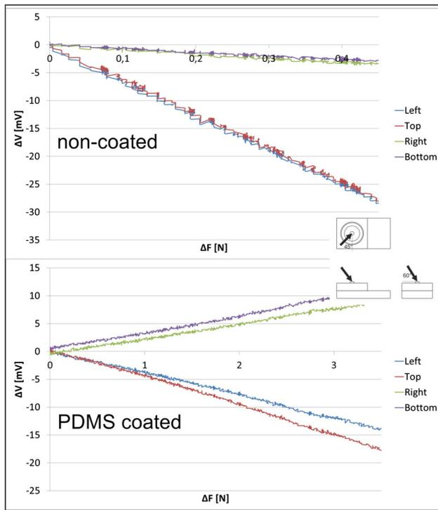
**Fig. 9** Sensitivity and response characteristics of the force sensing elements for load direction indicated by the inset. The sensor is exposed to load of  $X = 60^\circ$  and  $Y = 45^\circ$  direction. The same chip was measured with and without elastic coating
