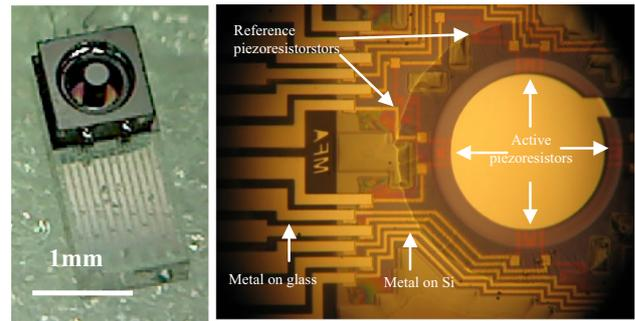
**Fig. 4** Optical views of glass bonded chip (left) and the same chip as looking from the glass side (right). The recessed ring facilitates uniformly shaped semi-sphere elastomer coating
