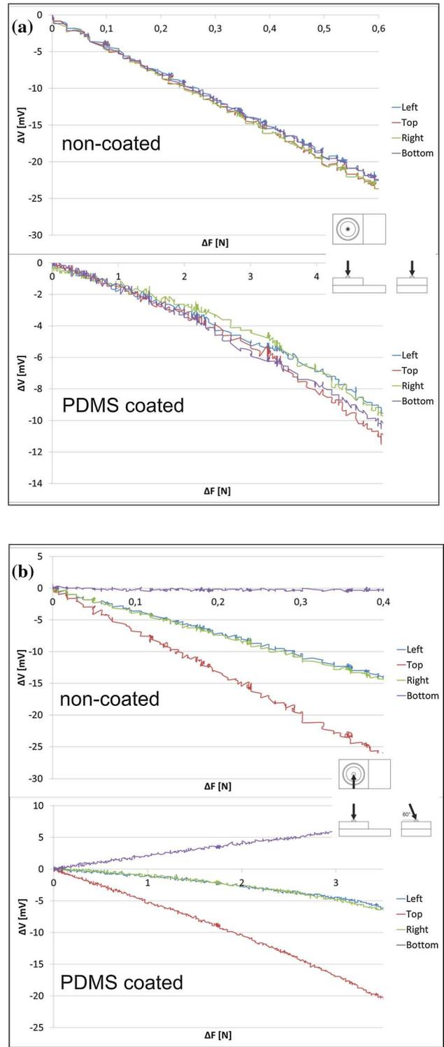
**Fig. 8** Sensitivity and response characteristics of the force sensing elements for load directions indicated by the insets. Perpendicular load (a) and 60° in Y direction (b). The same chip was measured with and without elastic coating
