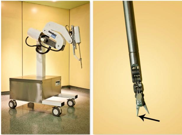
**Fig. 1** Elements of the surgery robots (FRK). Assembled robotic arm (left) and the laparoscopic head where the force sensors must be integrated (right)
