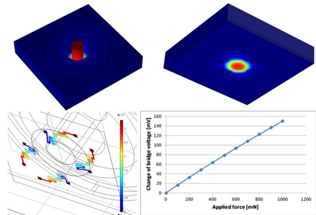
**Fig. 3** Coloured representation of the coupled FEM simulation: deformation and mechanical stress distribution of the membrane (top) and the four piezoresistors (bottom left). The calculated sensor signal for perpendicular load is also shown (bottom right). Membrane thickness is  $20 \mu\text{m}$
