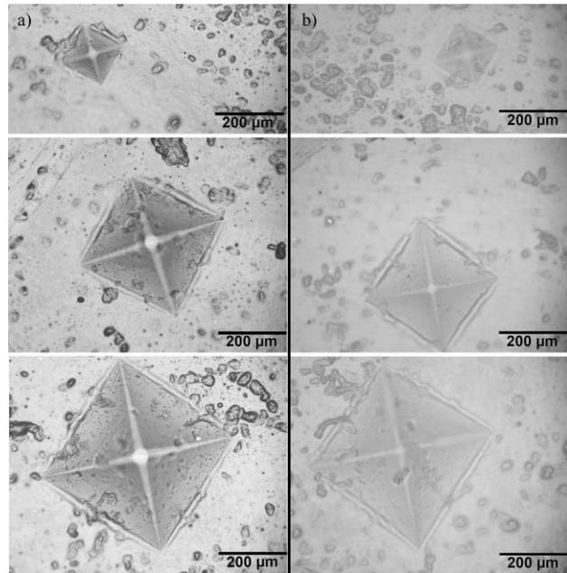
Figure 6. The impression on the RGD720 (a) and the RGD835 (b) materials at a loading force of 1 N (top), 6 N (middle) and 12 N (bottom)
