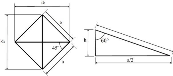
Figure 4. The impression of a Vickers indenter and its geometrical parameters [2]
