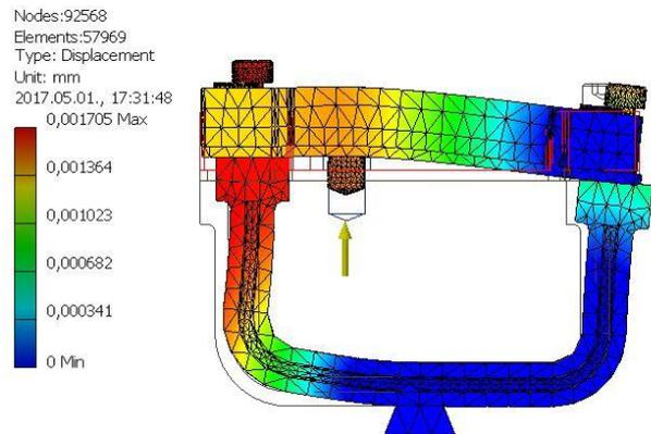
Figure 2. The finite element simulation results of the horse race track in an extreme position
