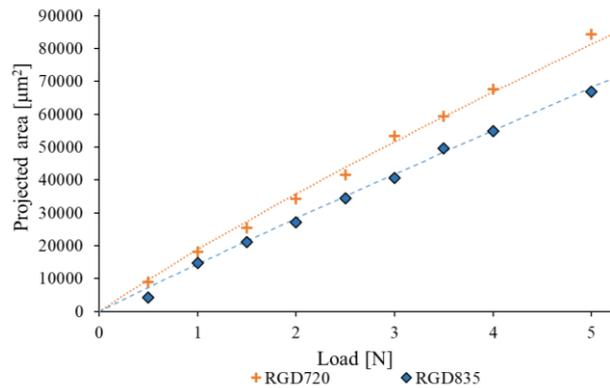
Figure 10. The projected area as a function of loading force, enlarged
