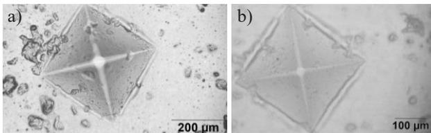
Figure 5. Pilling-up on the RGD720 (a) and sinking-in on the RGD835 material (b)
