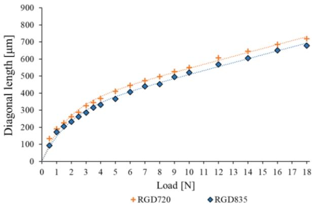
Figure 8. Average diagonals as a function of loading force
