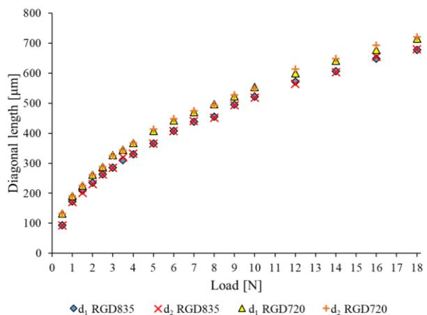
Figure 7. Comparison of the diagonals of impressions in both materials
