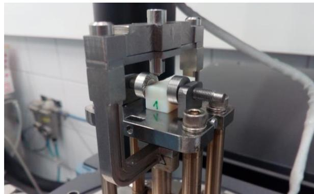
Figure 3. The fixture we designed and the gripped photopolymer specimen
