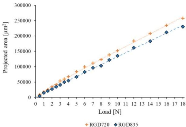
Figure 9. Projected area as a function of loading force
