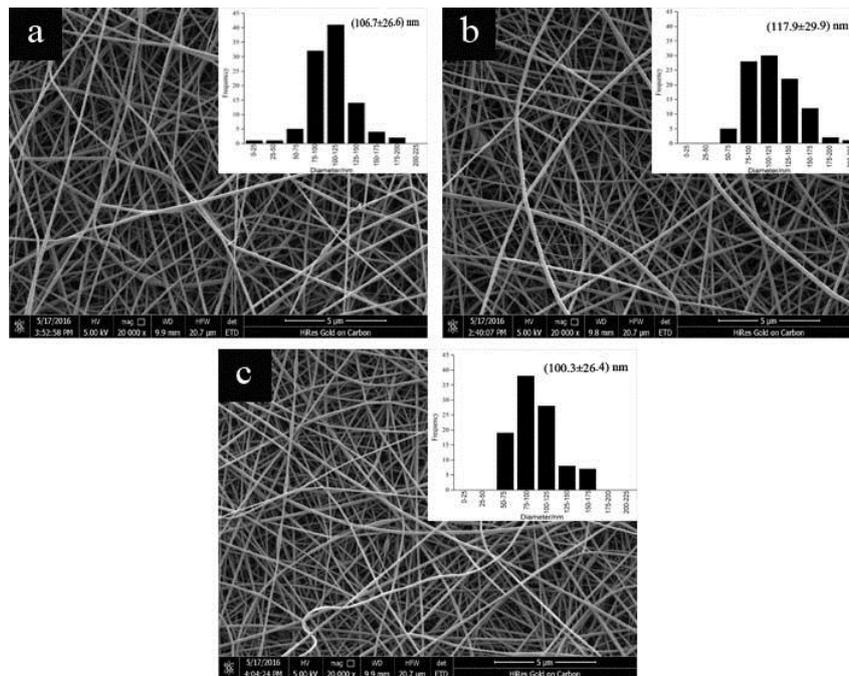
**Fig. 5** Morphology and diameter distribution of nanofibers obtained at different traction
