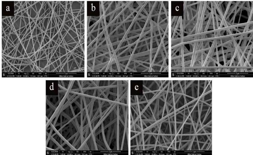
**Fig. 6 Morphology of electrospun nanofibers from different kinds of and differently charged yarns: (a) U-SSCY-40; (b) G-SSCY-40; (c) G-SFY-40; (d) G-PFY-40; (e) G-PFY-65 (scale bar indicates 5  $\mu\text{m}$ )**
