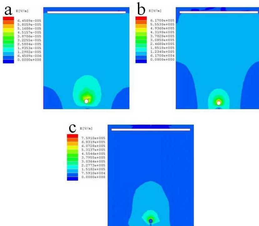
**Fig. 9 FEA of electrostatic field intensity around the yarn (the upper body is the collector**
