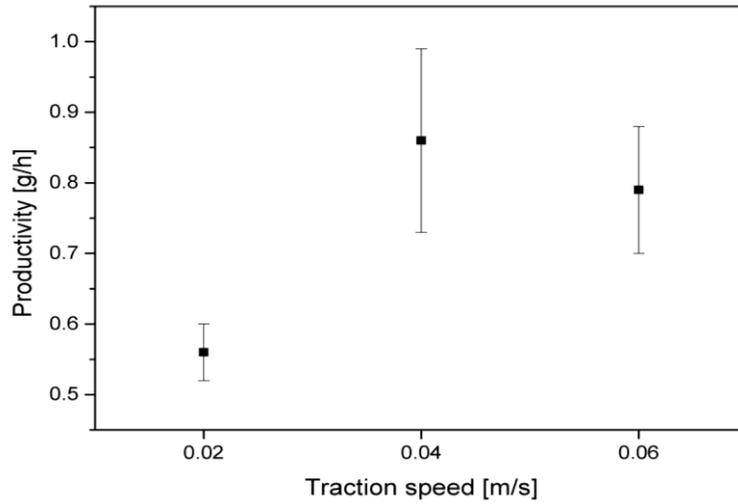
**Fig. 4** Productivity at different traction speeds
