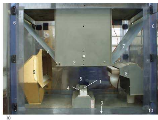
Figure 1. Electrospinning setup used to collect nanofibers on the surface of reinforcing materials. 1: rotary electrode, 2: grounded plate electrode, 3: high-voltage power supply, 4: polymer solution, 5: fiber formation space, 6: rollers, 7: moving belt collector, 8: air inlet, 9: air outlet, 10: chamber.
