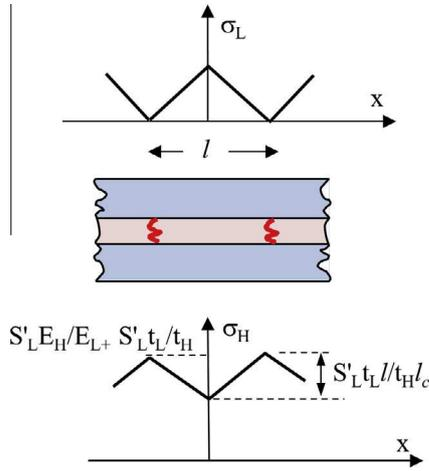
**Fig. 5.** A representative volume element with length of  $l_c \geq l \geq l_c/2$ . (For interpretation of the references to colour in this figure legend, the reader is referred to the web version of this article.)
