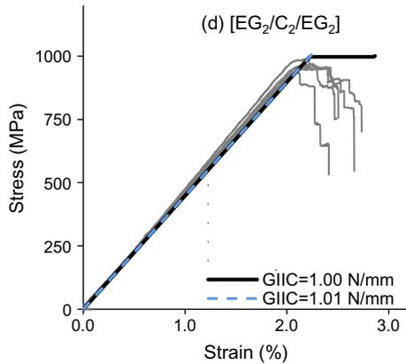
**Fig. 10.** The predicted stress–strain curve of  $[EG_2/C_2/EG_2]$  with two different values of 1.00 and 1.01 N/mm for  $G_{IIIC}$ . (For interpretation of the references to colour in this figure legend, the reader is referred to the web version of this article.)
