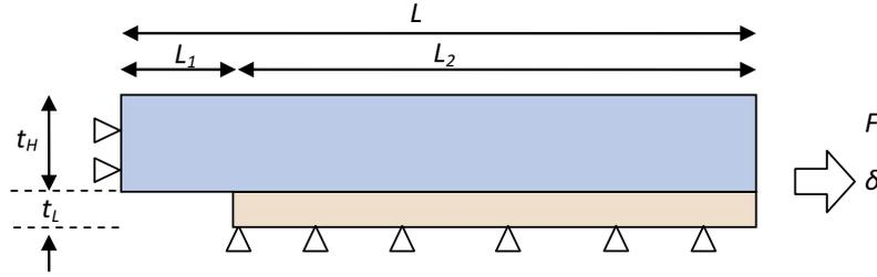
**Fig. 6.** Representative Volume Element (RVE) of a UD hybrid to predict delamination. (For interpretation of the references to colour in this figure legend, the reader is referred to the web version of this article.)
