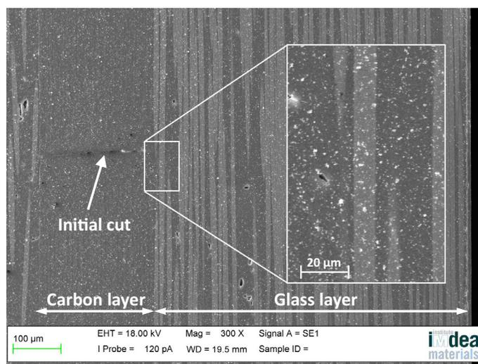
**Fig. 3.** Typical scanning electron micrograph showing the alumina particle coated surface of the tensile specimens. (Light grey bands are individual glass fibres, bright white spots are the alumina particles.)
