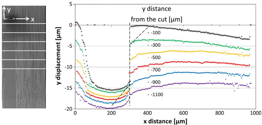
Fig. 10. Plots of  $y$  displacements across the thickness ( $x$  direction) of the hybrid layers at  $428 \text{ MPa}$  stress level with a schematic showing the positions of the un-deformed lines at various  $y$  coordinates.
