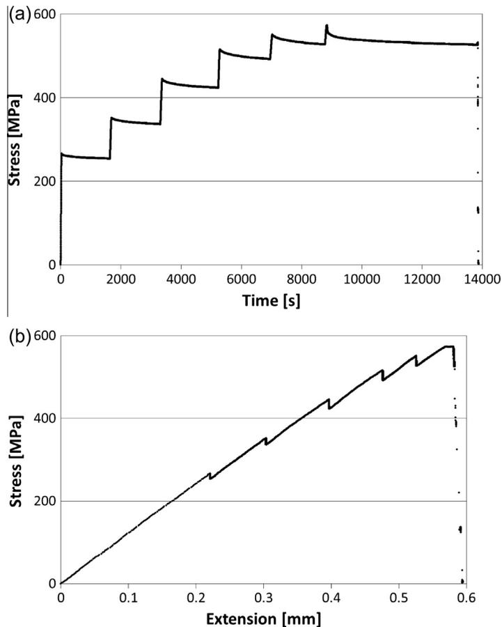
**Fig. 5.** Typical (a) load-time and (b) load-extension graphs of an in-situ SEM tensile test. (Test speeds: 0.5 mm/min up to the first step, 0.1 mm/min up to the fourth step and 0.05 mm/min up to the last step.)
