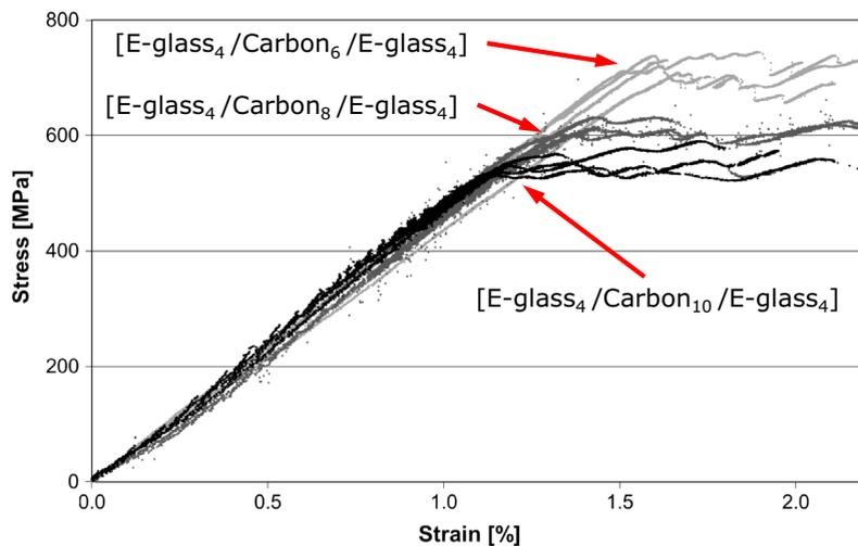
Fig. 2. Tensile test results summary of  $1.5 \times 1.5 \times 30$  mm<sup>3</sup> nominal size UD glass/carbon–epoxy hybrid specimens with a single cut through the central carbon/epoxy layer.
