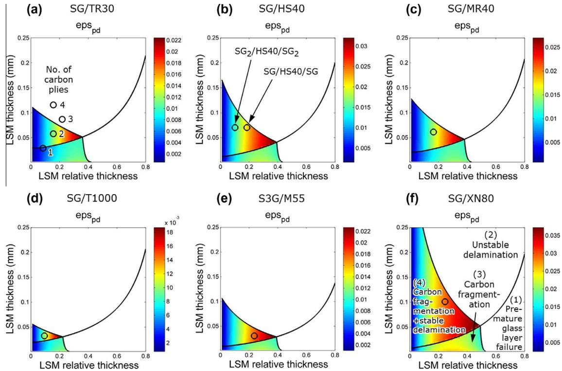
Fig. 2. Damage mode maps of the designed material combinations with S-glass and various carbon plies ( $\epsilon_{ps\_pd}$  – pseudo-ductile strain, LSM – low strain material (i.e. carbon), part f) indicates four regions of the map with their associated failure processes).
