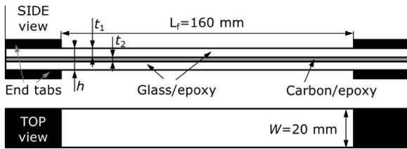
Fig. 3. Schematic of the specimen geometry.
