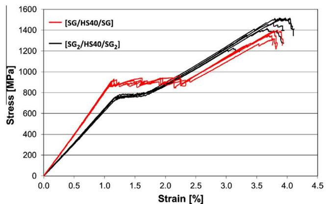
Fig. 5. Tensile stress–strain graphs of S-glass/HS40 carbon configurations.
