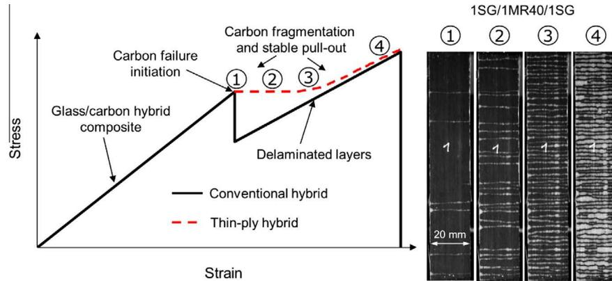
**Fig. 1.** Schematic of the stress–strain response of conventional and thin-ply interlayer hybrid composites and typical appearance of thin-ply hybrid specimens at successive damage phases (dark areas show bonded, light areas show damaged glass/carbon interface through the translucent outer glass layer).
