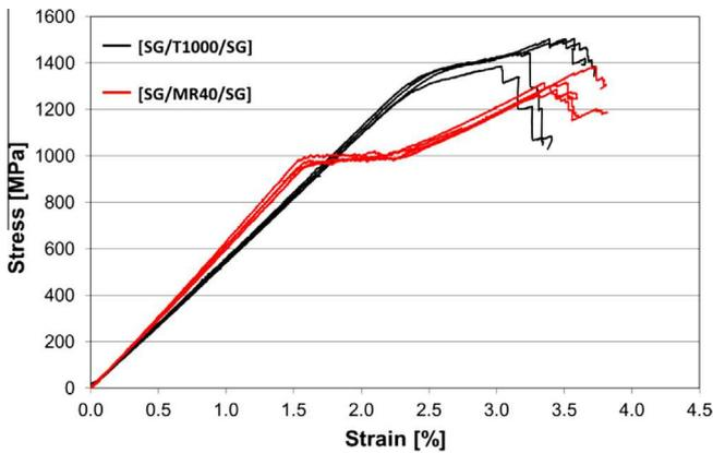
Fig. 6. Tensile stress–strain graphs of S-glass/IM carbon configurations.
