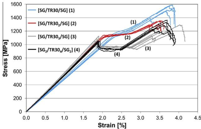
Fig. 4. Tensile stress–strain graphs of S-glass/TR30 carbon configurations.
