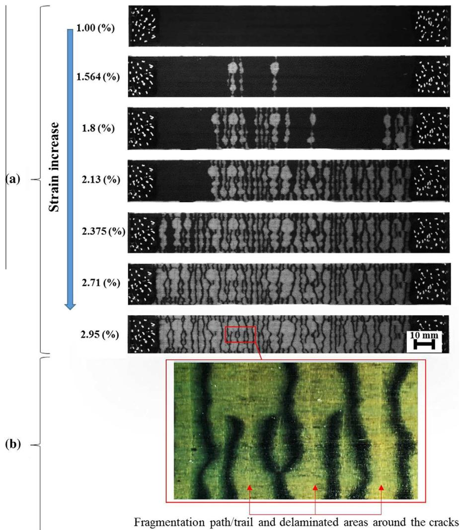
**Fig. 16.** (a) The appearance of a typical MR40/S-glass specimen at different strains during the tensile test and (b) Microscopy pictures with higher zoom (the fragmentation path and delaminated areas around the cracks). (For interpretation of the references to colour in this figure legend, the reader is referred to the web version of this article.)
