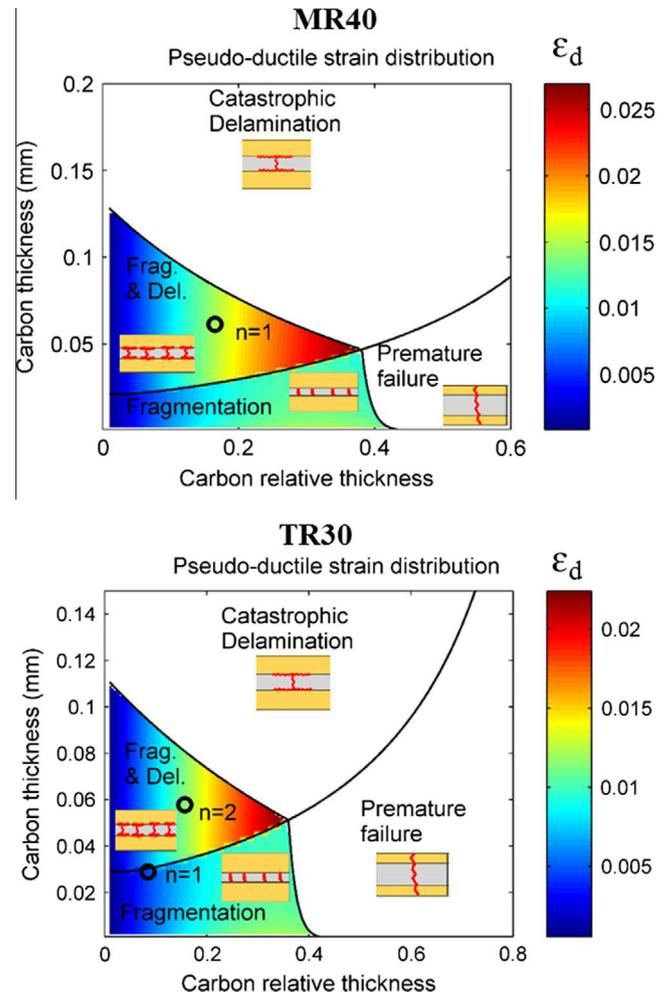
**Fig. 2.** Distribution of pseudo-ductile strain for  $[G_1/C_n/G_1]$  laminates made with MR40 and TR30 carbon, where  $(n = 1-3)$ . (For interpretation of the references to colour in this figure legend, the reader is referred to the web version of this article.)
