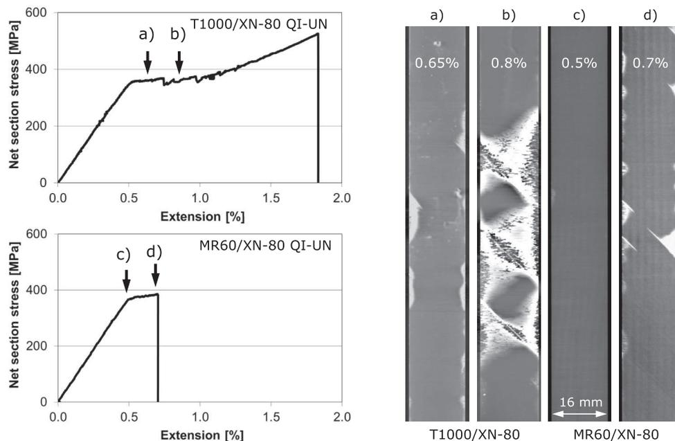
**Fig. 6.** X-ray CT scans showing inter-sublaminar damage in QI-UN laminate specimens after tests interrupted at specific strains: (a) T1000/XN-80 QI-UN 0.65% (at plateau, before any stress-drop), (b) T1000/XN-80 QI-UN 0.8% (after the first stress-drop), (c) MR60/XN-80 QI-UN 0.5% (at knee point), (d) MR60/XN-80 QI-UN 0.7% (at plateau, before any stress-drop).
