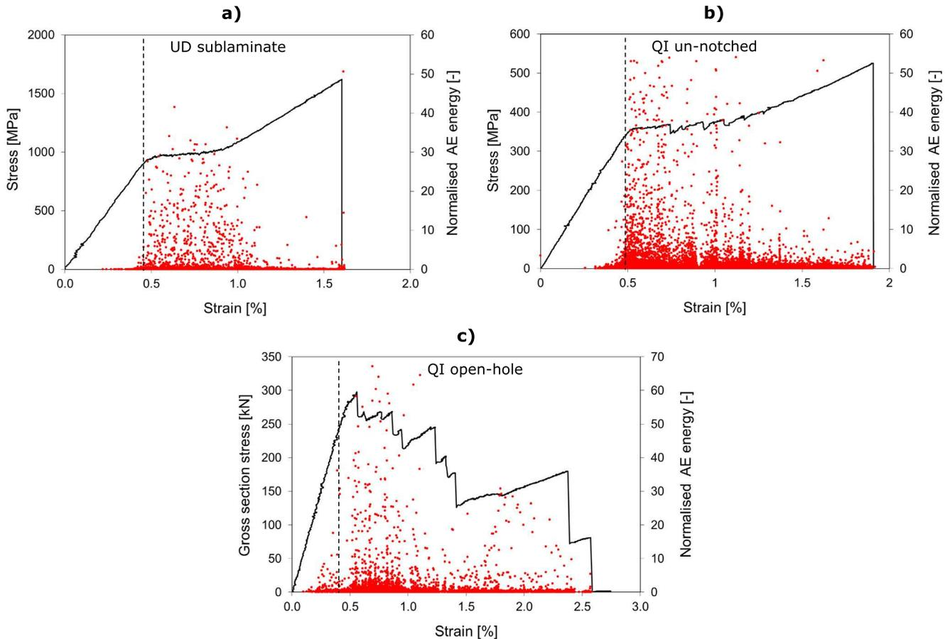
**Fig. 11.** Graphs showing typical plots of the acoustic event energy normalised to the average AE energy of each test for T1000/XN-80 specimens: (a) UD sublaminates, (b) QI un-notched and (c) QI open-hole specimen. Dashed lines highlight the damage initiation. (For interpretation of the references to colour in this figure legend, the reader is referred to the web version of this article.)
