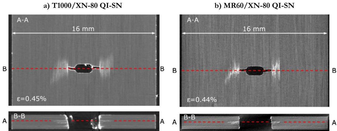
**Fig. 9.** Full width X-ray CT scans of different type notched specimens after tests interrupted before any stress-drop at the overall strains indicated on the scans. Top view scans show the damage in one of the  $0^\circ$  sublaminates. (For interpretation of the references to colour in this figure legend, the reader is referred to the web version of this article.)
