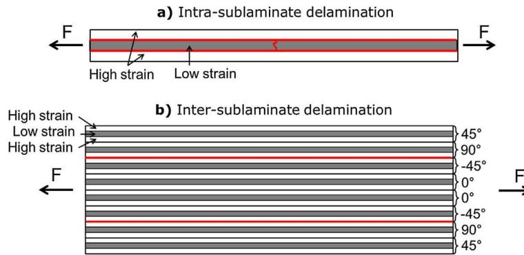
**Fig. 2.** Two levels of delamination in multi-directional hybrid laminates indicated by red lines. (For interpretation of the references to colour in this figure legend, the reader is referred to the web version of this article.)
