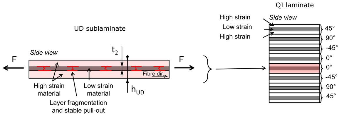
**Fig. 1.** Schematic showing the sublaminate concept for multi-directional composite plates. (For interpretation of the references to colour in this figure legend, the reader is referred to the web version of this article.)
