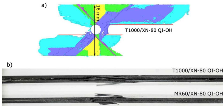
**Fig. 10.** (a) Post-processed X-ray CT scan showing delamination and splitting of a T1000/XN-80 QI-OH specimen unloaded from 0.58% strain after the first stress-drop and (b) post mortem photographs of QI-OH specimens (edge view). (For interpretation of the references to colour in this figure legend, the reader is referred to the web version of this article.)
