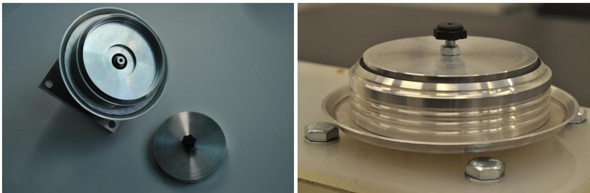
Figure 3. The machined spinneret
