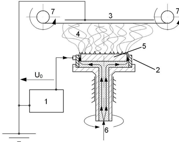
Figure 1: Scheme of the novel electrospinning method. 1: High voltage power supply, 2: Electrode (sharp edge), 3: Collector (grounded aluminum plate), 4: Forming nanofibers, 5: Blunt cylindrical part (*i.e.* lid), 6: Solution feed, 7: Traction of the textile collector substrate
