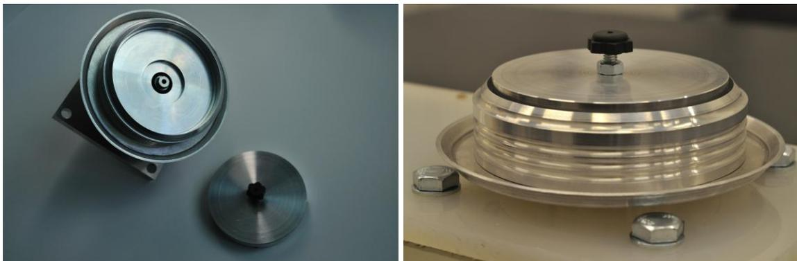
Figure 3. The machined spinneret
