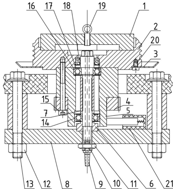
Figure 2. Engineering draft of the spinneret, 1: lid, 2: spinneret, 3: overflow collecting plate, 4: belt drive, 5-7: bearing holders, 8: base platform, 9: solution inlet, 10: shaft, 11-13: hex nuts and screws, 14: deep groove roller bearing, 15: holder screws, 16: deep groove roller bearing, 17-18: sealing and holder, 19: lid screw, 20: screws, 21: carbon brush
