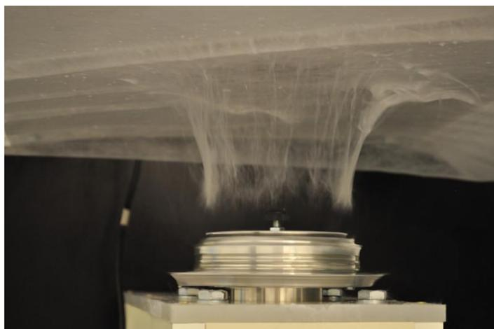
Figure 4. Electrospinning device at work
