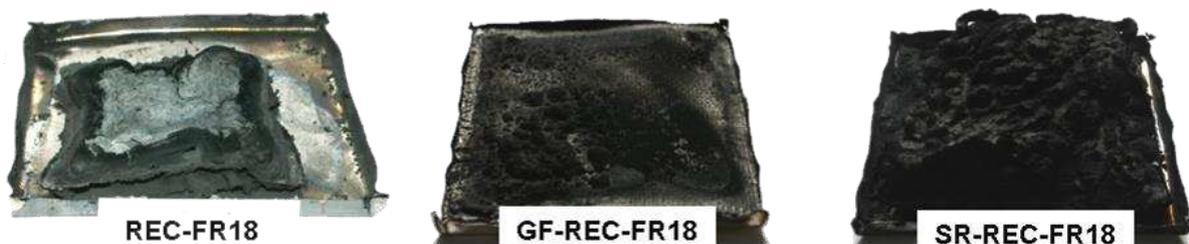
**Fig. 6. Photographs taken of the charred residues of flame retarded samples obtained after combustion in Mass Loss type Cone Calorimeter**
