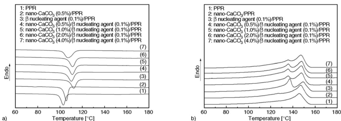
Figure 1. (a) DSC cooling and (b) heating curves of PPR and its composites
