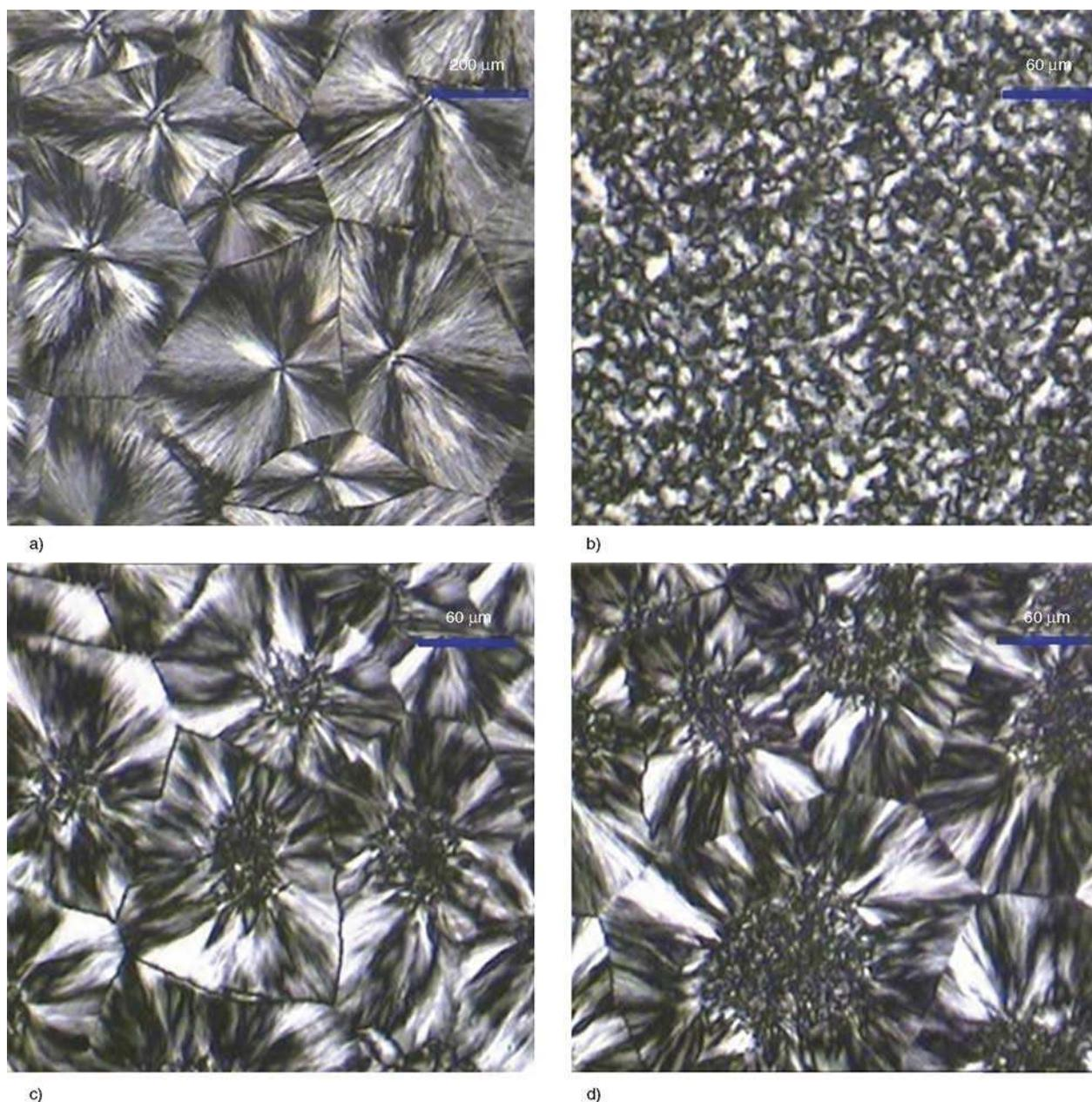
**Figure 4.** Optical micrographs of (a) PPR, (b) nano- $\text{CaCO}_3$  (0.5 wt%)/PPR, (c)  $\beta$  nucleated PPR (content of  $\beta$  nucleating agent: 0.1 wt%) and (d) nano- $\text{CaCO}_3$  (0.5 wt%)/ $\beta$  nucleated PPR (content of  $\beta$  nucleating agent: 0.1 wt%). Crystallization conditions:  $130^\circ\text{C}$ , 16 h.
