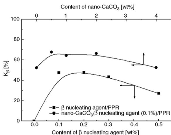
**Figure 3.** Relative amount of  $\beta$  crystal,  $K_\beta$ , of PPR as a function of contents of  $\beta$  nucleating agent and nano- $\text{CaCO}_3$
