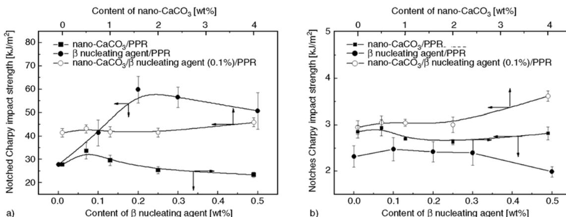
**Figure 6.** Notched Charpy impact strength of PPR as a function of contents of  $\beta$  nucleating agent and nano-CaCO<sub>3</sub>. Test temperature: (a) 23°C and (b) -10°.
