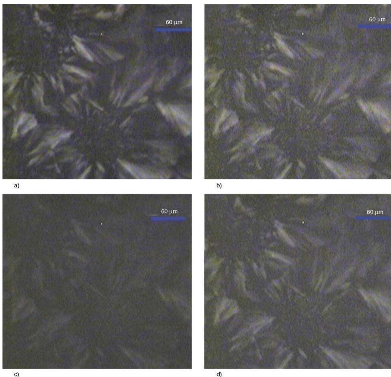
**Figure 5.** Optical micrographs showing melting process of  $\beta$  nucleated PPR (content of  $\beta$  nucleating agent: 0.1 wt%) after crystallization at 130°C for 16 h. Heating rate: 0.1°C/min. (a) 132°C, (b) 137°C, (c) 142°C and (d) 148°C.
