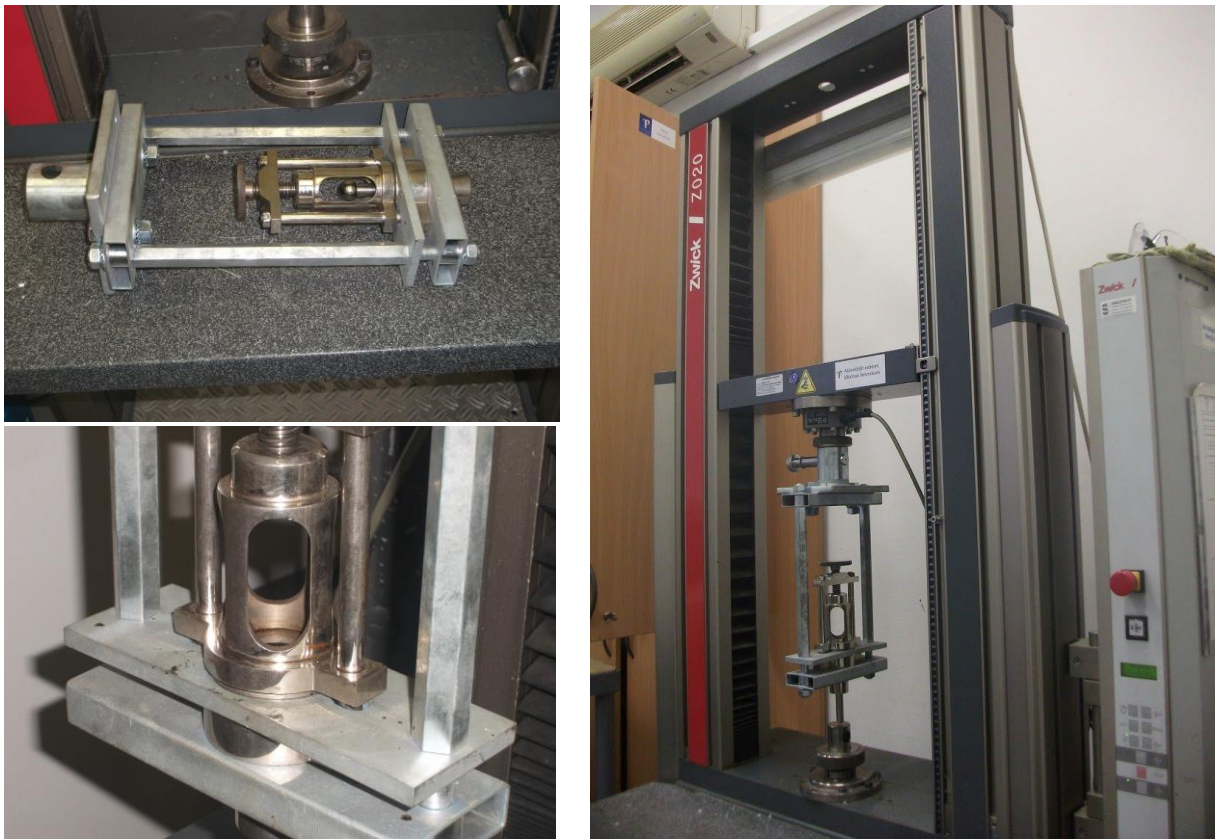
Figure 3: Bursting equipment (on the left side) and as it is installed on Zwick Z020 testing machine (on the right side)
