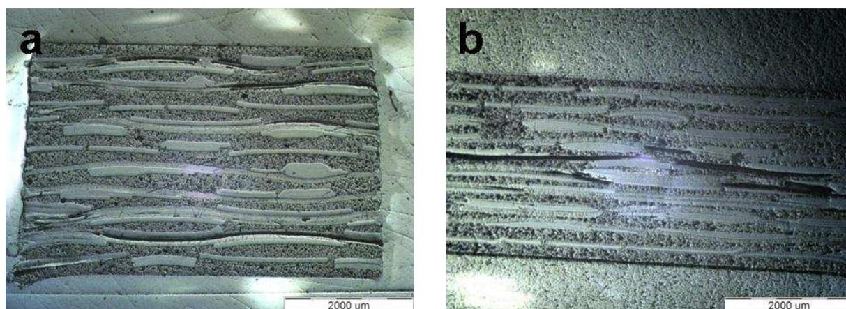
**Figure 7 Light microscopic photographs of the cross section of multilayer SRCs reinforced with (a) non-treated and (b) heat treated PP fabrics**
