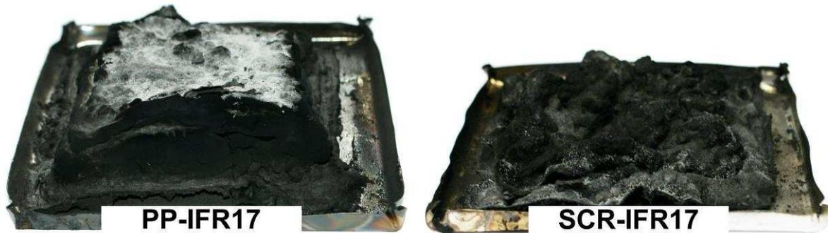
**Figure 3 Charred residues of 17 wt% IFR containing samples obtained after cone calorimetric tests**
