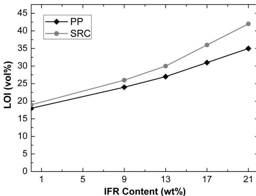
**Figure 1 LOI as a function of IFR content in case of PP based compounds and SRCs**
