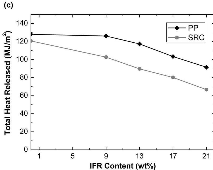
**Figure 4 Results of the comparative combustion tests under 50 kW/m<sup>2</sup> irradiation of conic heater: a) time to ignition, b) residual mass and c) total heat released**
