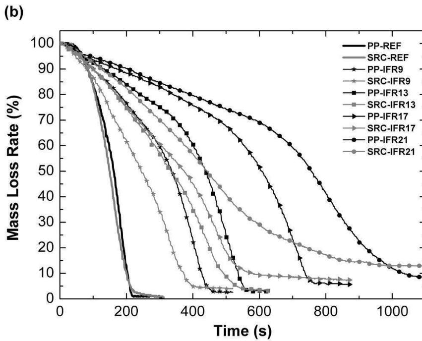
Figure 2 Comparison of a) heat release rate curves and b) mass loss rate curves recorded during the combustion of simple compounds and self-reinforced composites with identical flame retardant contents
