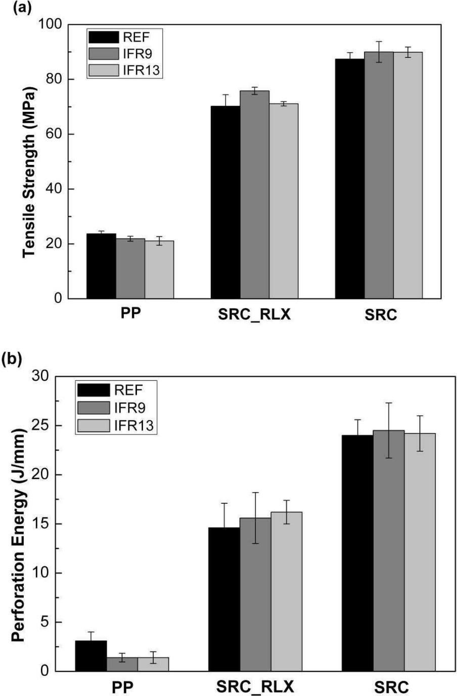
Figure 5 (a) Tensile strength and (b) perforation energy of PP compounded mixtures, SRCs and relaxed SRCs with identical IFR contents
