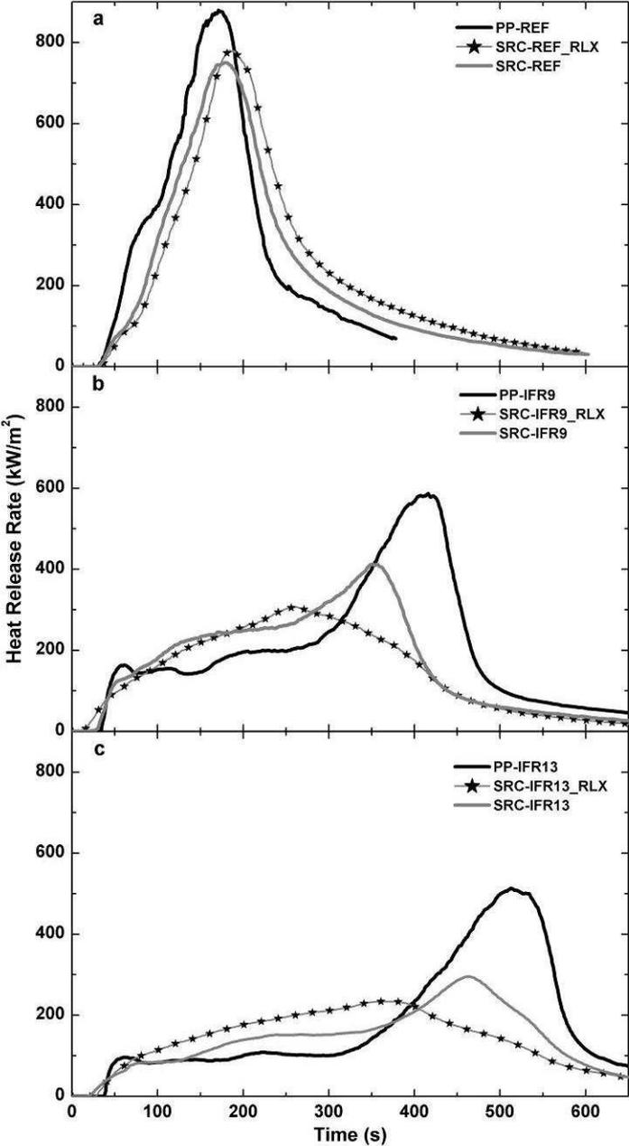
**Figure 6 Heat release rate curves recorded during the burning of flame retarded simple compounds, high-performance and relaxed SRCs with IFR content of 0, 9 and 13 wt%, respectively**
