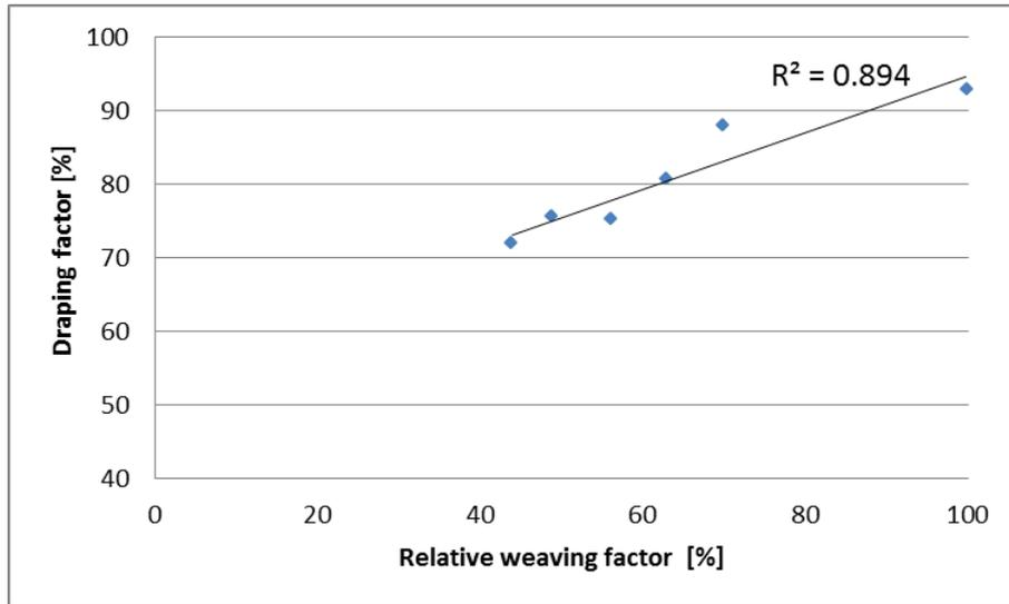
Figure 4: Drape coefficient depending on the relative weaving factor
