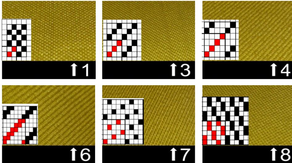
Figure 1: Weaving type of fabrics
