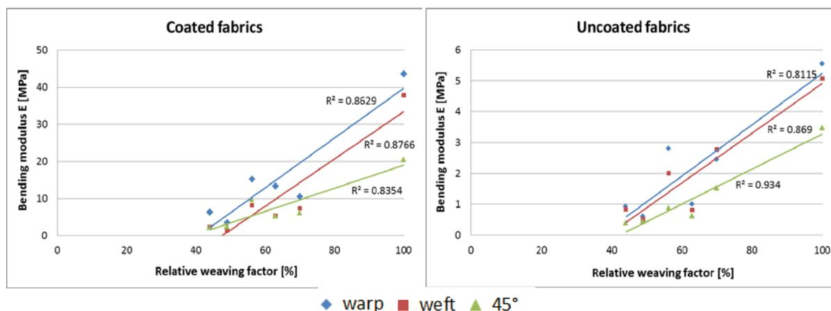
*Figure 6: Bending modulus of the coated and uncoated fabrics in different directions depending on relative weaving factor measured by Flexometer*
