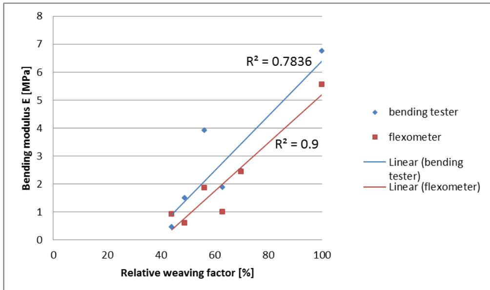
Figure 5: Bending modulus of the uncoated fabrics depending on relative weaving factor measured by Sylvie Bending Tester and Flexometer
