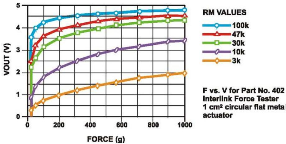
Figure 5. Output characteristic of sensors v reference<sup>4</sup>
