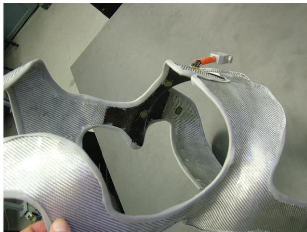
Figure 14. The composite corsette with the connector and built sensors
