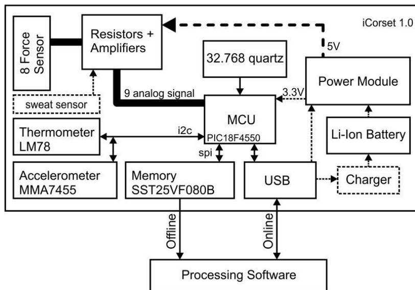
Figure .6 iCorset 1.0 block diagram
