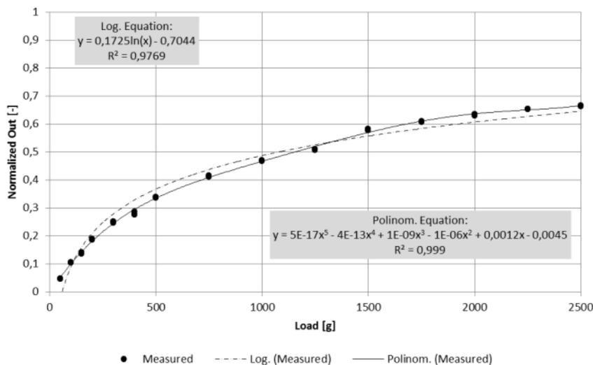
Figure 10. Normalized output as a function of pressure
