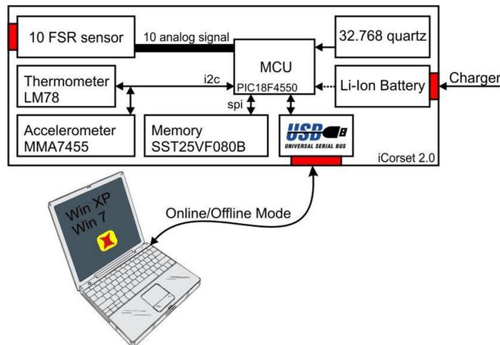
Figure.7. iCorset 2.0 block diagram
