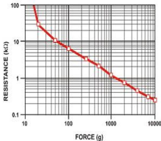
Figure 3. FSR sensor characteristic reference<sup>4</sup>
