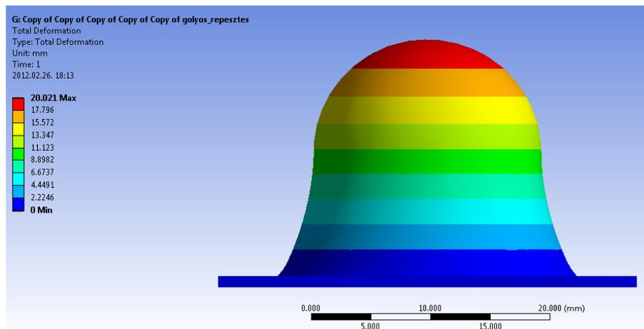
Figure 17: Total deformation of the FEM model
