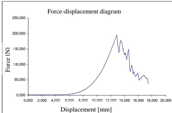
Figure 2: Typical curve of several step splitting
