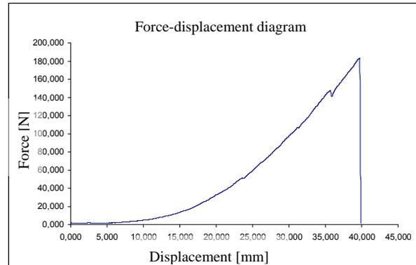
Figure 3: Typical curve of one step splitting
