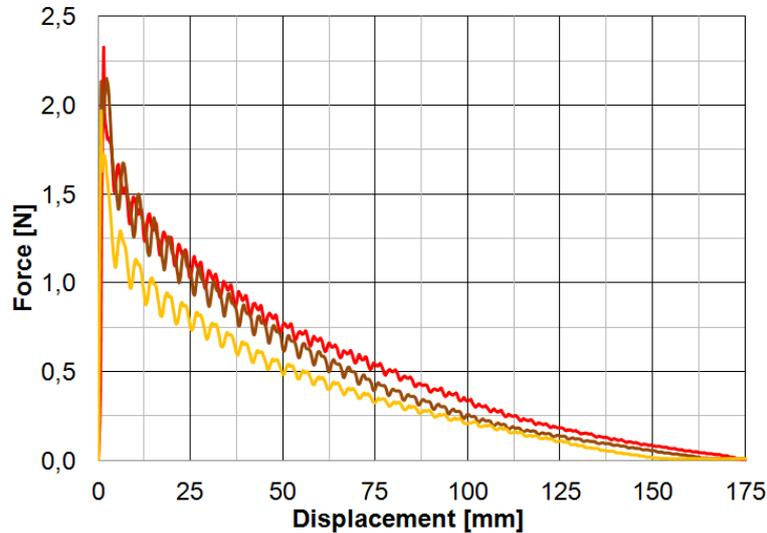
Figure 6. Brief results of the yarn pull-out tests
