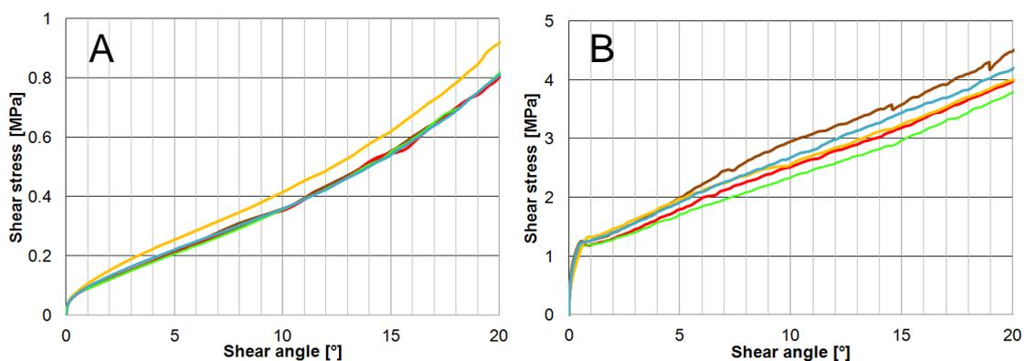
Figure 5. Shear diagrams measured with the aid of the designed apparatus. Samples cut at: A: 0° direction B: 45° direction
