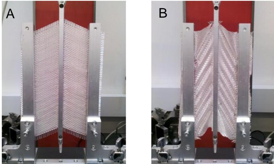
Figure 4. Deformation of the sample at shear test. A: 0° direction, B: 45° direction
