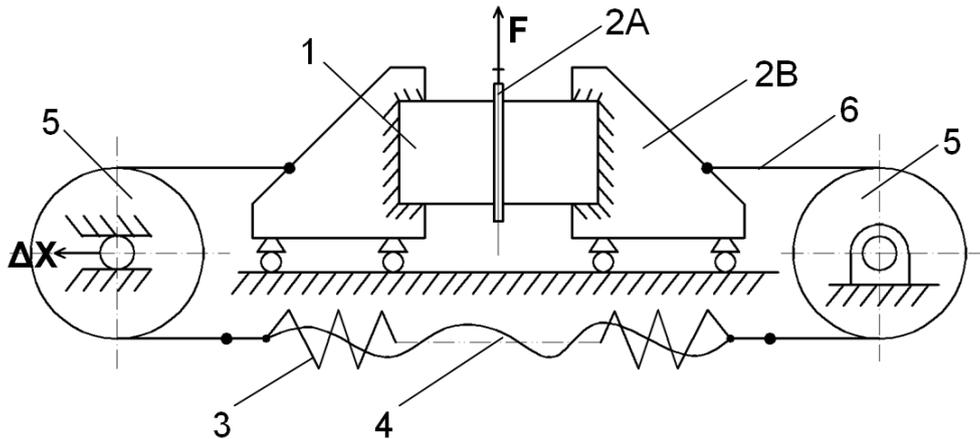
**Figure 1.** The schematic draft of the apparatus. 1: textile specimen, 2A & 2B: grippers, 3: steel spring, 4: HOPE yarn, 5: rollers with bearing, 6: rope
