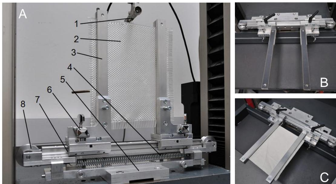
**Figure 3.** Apparatus for determining shear properties of textiles at yarn pull-out test. A: beginning of test, B: tilted to horizontal position, C: specimen gripping, 1: clamping unit connected to the crosshead of the tensile tester, 2: test specimen, 3: clamps, 4: pretension spring, 5: motherboard, 6: gears for adjusting pretension, 7: linear bearing, 8: rollers with bearings
