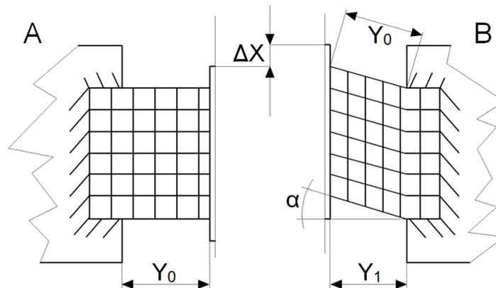
**Figure 2.** The specimen at shear test. A: before test, B: deformation during test
