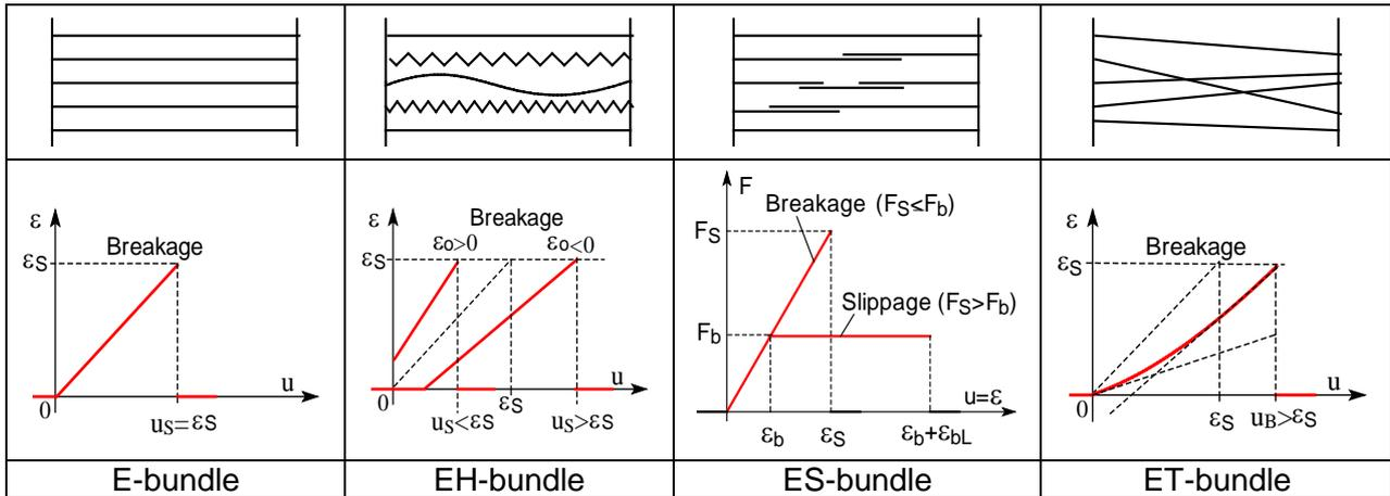
**Figure 1.** Structural scheme of the idealized fiber bundle cells and relationship between the strains of single fibers and FBCs [4]
