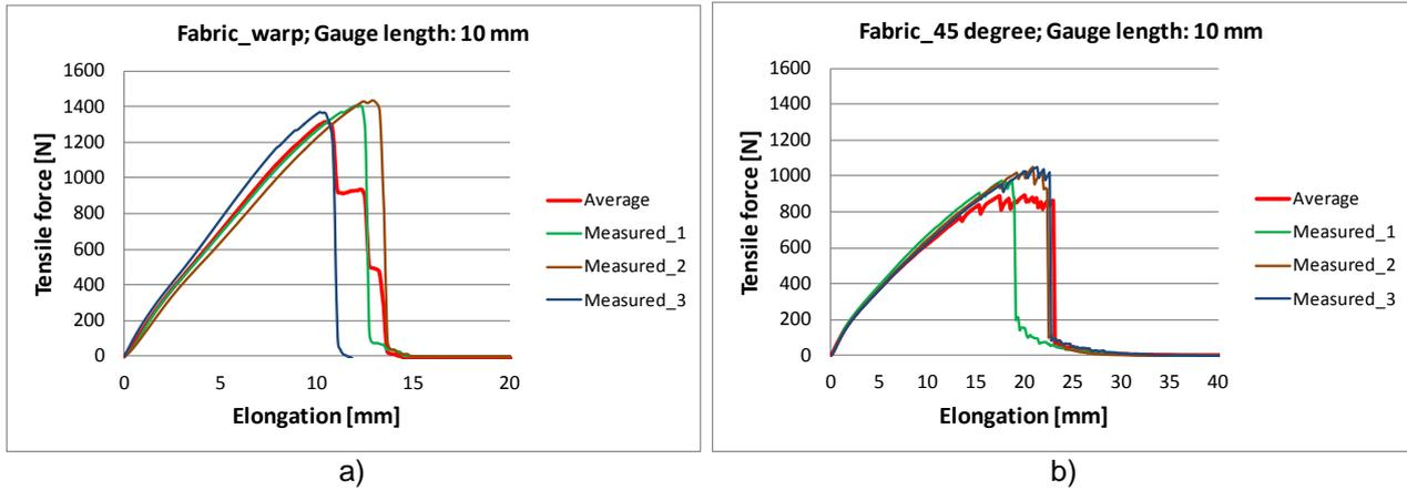
**Figure 7.** Tensile test measurements performed at gauge lengths 10 mm on fabric samples cut in warp (a) and 45° (b) directions
