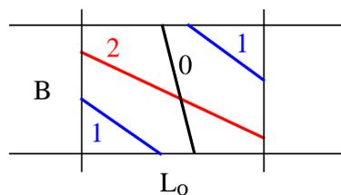
**Figure 3.** Yarn positions gripped at zero-, one-, and two-ends in a fabric sample
