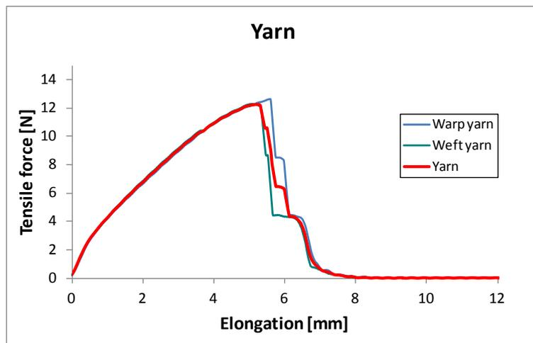
Figure 6. Averaged tensile load versus elongation curves of the warp and weft yarns and their average
