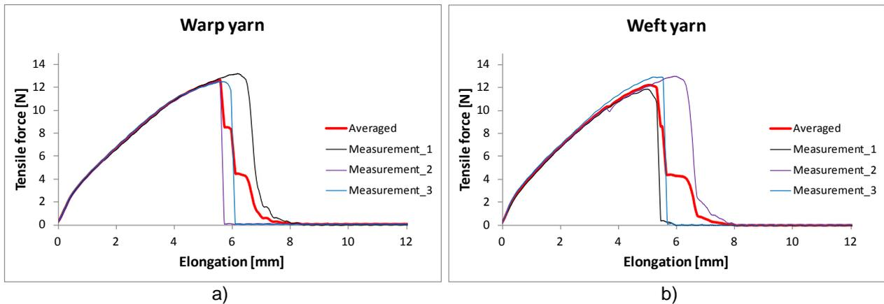
Figure 5. Tensile test measurements performed at gauge lengths 10 mm on warp (a) and weft (b) yarn samples
