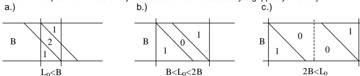
**Figure 4.** Bundle structure of a fabric sample in 45° direction at different gauge lengths
