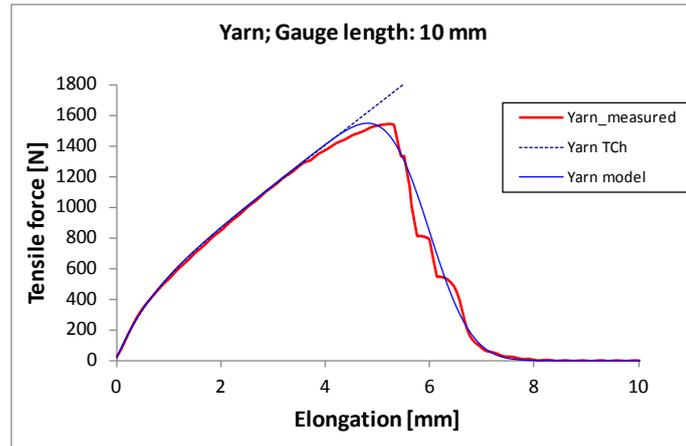
**Figure 9.** The averaged force-elongation curve of 3 measurements performed at gauge lengths 10 mm on yarn samples and the FBC-model-curve
