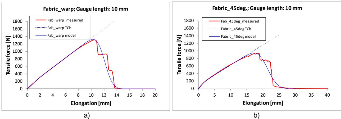
**Figure 10.** The averaged force-elongation curves of 3 measurements performed at gauge lengths 10 mm on fabric samples in warp and 45° directions and the FBC-model-curves
