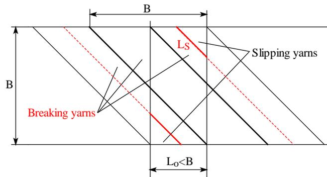
**Figure 5.** Bundle structure of a fabric sample in 45° direction if the gauge length is small and the adhesion between yarns is rather large
