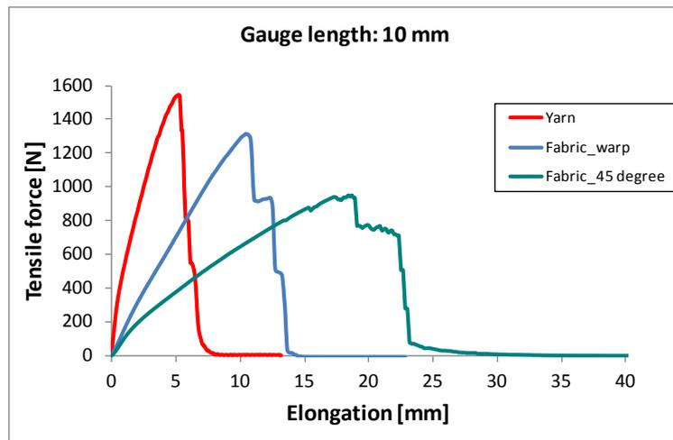
**Figure 8.** Tensile test measurements performed at gauge lengths 10 mm on yarn and fabric samples, the latter in warp and 45° directions
