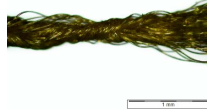
Figure 6 The structure of yarn in optical microscope
