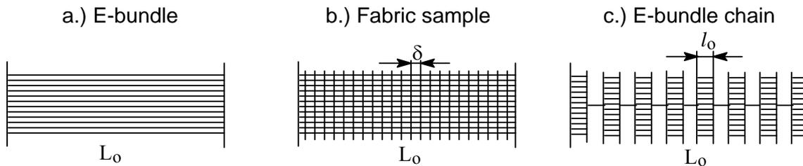
Fig. 8 E-bundle (a), a fabric sample cut out in main direction (b) and E-bundle chain (c) as the model of the sample
