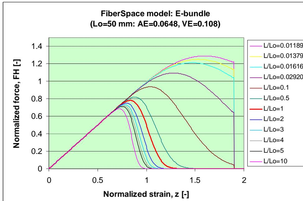
Fig. 10 Normalized expected force-strain curves of E-bundles with different relative lengths ( $L/L_0$ )
