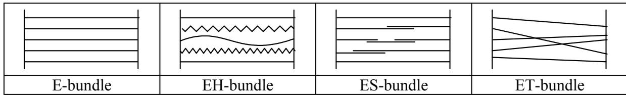
Fig. 1 Structural scheme of the idealized fiber bundle cells
