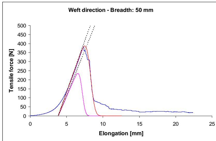
Fig. 12 Measured and averaged force-elongation curve (blue line), shifted E-bundle curve (lilac line), and the transformed model curve (red line) for samples cut out of weft direction
