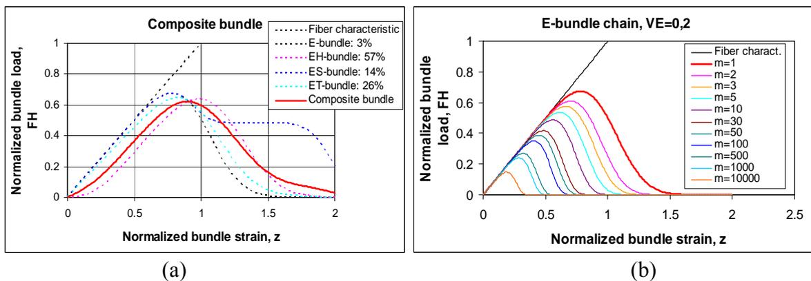
Fig. 5 Normalized mean force-strain curves of parallel (a) and serial (b) connected FBCs
