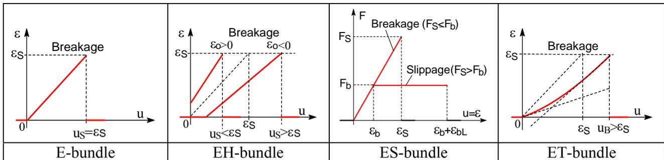
Fig. 2 Relationship between the strains of single fibers and FBCs
