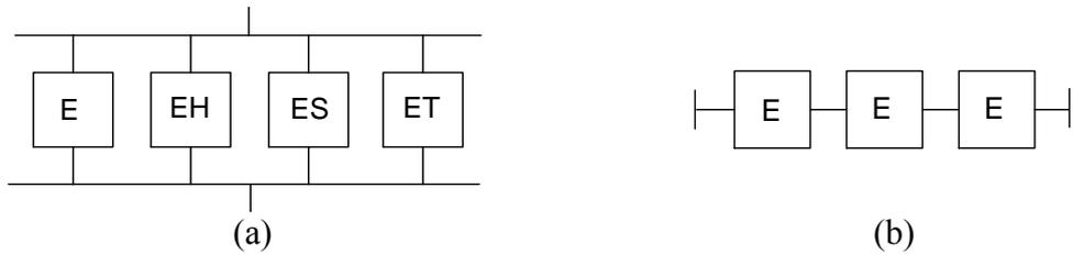
Fig. 4 (a) Parallel and (b) serial connections of FBCs
