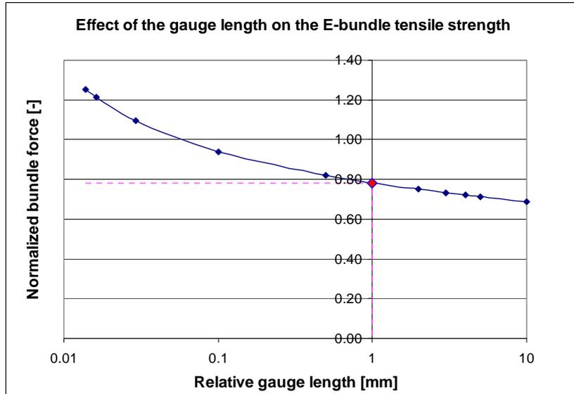
Fig. 11 Peak values of E-bundles versus relative yarn length in logarithmic scale
