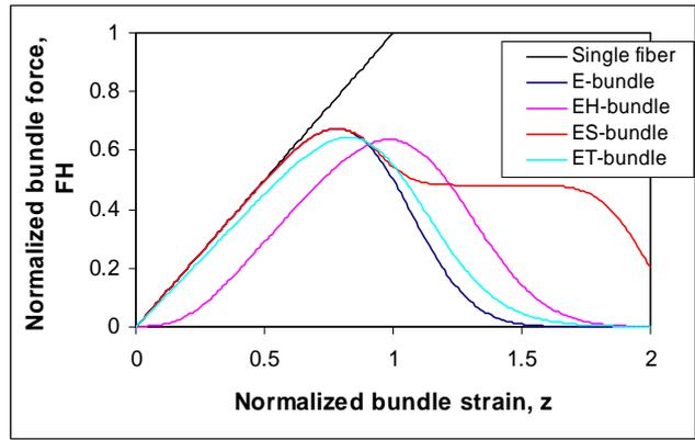
Fig. 3 Expected value of typical normalized force-strain curves of the FBCs
