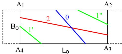
Fig. 7 Classification of yarns according to their gripping position
