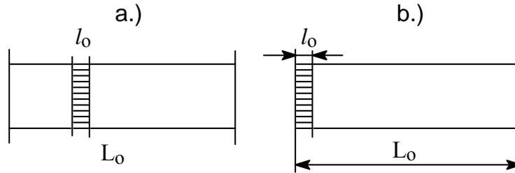
Fig. 9 Fabric sample as the serial connection of a single breaking E-bundle and an elastic part
