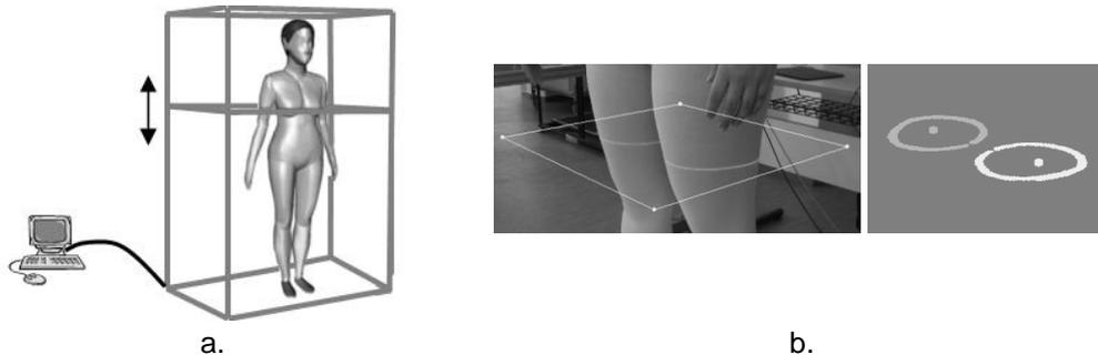
**Figure 2:** a) The scanner structure; b) One shot and the reconstructed point set from four side shot
