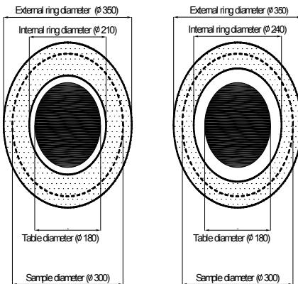
**Figure 2** Dimensions of rings
