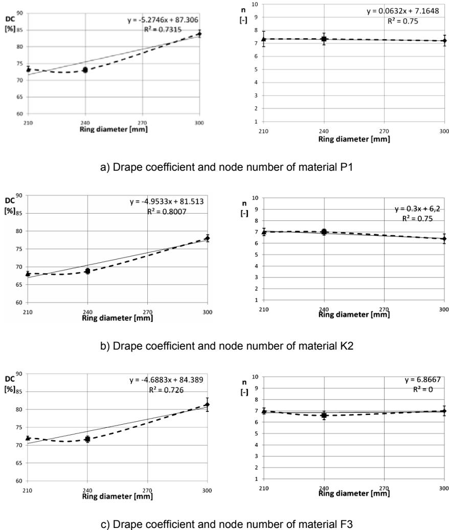
**Figure 5** Drape coefficients (DC) and node numbers (n) of three different materials (P1, K2, F3) with no ring (300 mm ring diameter) and with two different rings (240 and 210 mm diameter)
