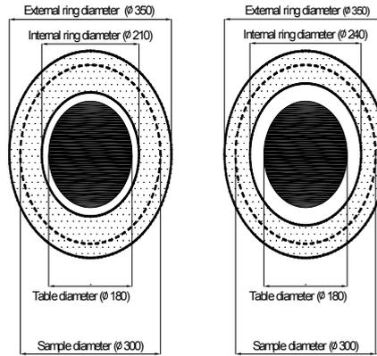
**Figure 2** Dimensions of rings
