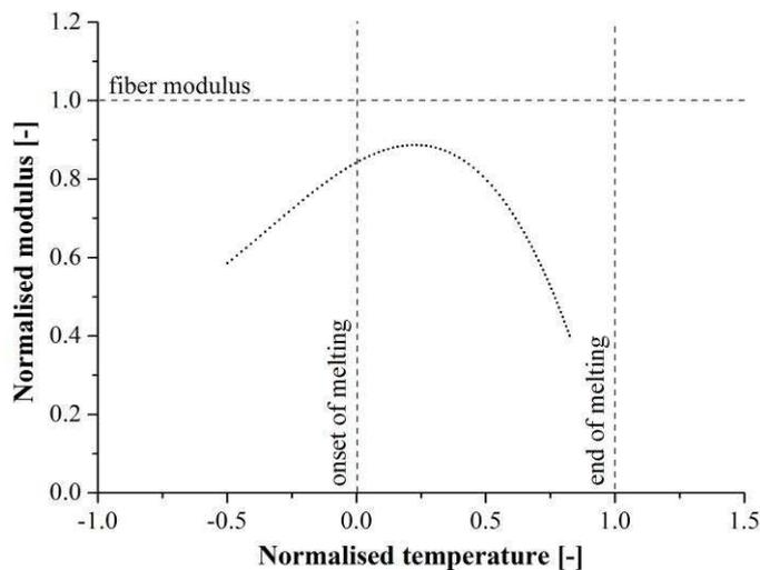
**Figure 5** Normalized modulus vs. normalized temperature chart for hot compacted semicrystalline polymer fibers, schematically. Notes: tensile moduli of the compacted fibers are normalized as a proportion of the initial fiber moduli and the compaction temperatures as a fraction of the total melting temperature interval of the fibers, i.e.  $= (T_{\text{compaction}} - T_{\text{onset}}) / (T_{\text{end of melting}} - T_{\text{onset}})$ . These temperatures are indicated in Figure 4 [82]
