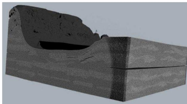
**Figure 8** Three-dimensional (3D) picture of an ultrasonic welding seam (overlapped) in a PP-based SPC revealed by X-ray micro computed tomography. Notes: the reinforcing iPP (ca. 40 wt%) in woven fabric form is well discernible. The seam thickness is about 1.5 mm.
