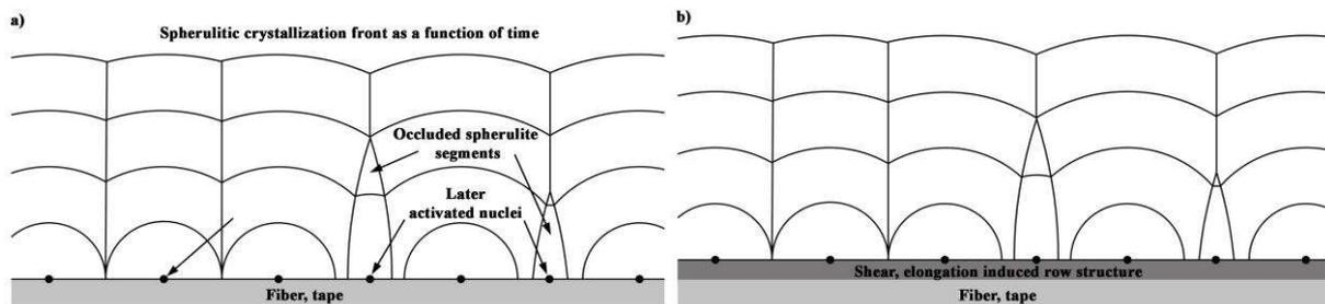
**Figure 3** Columnar crystallization caused by heterogeneous (transcrystallization, a) and homogeneous, row-induced nucleation (cylindrite formation, b), schematically. Note: structure of the cylindrite may be far more complex when the nuclei generate the spherulitic growth of different polymorphs [62].
