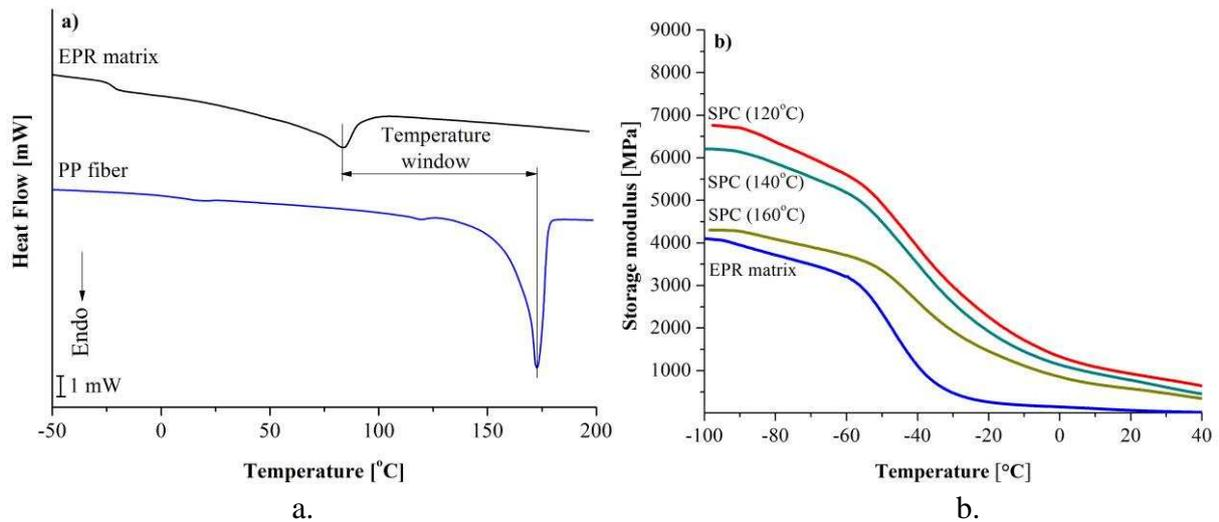
**Figure 7** DSC melting of a thermoplastic EPR matrix and reinforcing iPP fiber (a), and DMA traces of the corresponding injection-molded SPC as a function of the molding temperature (b). Note: the chopped iPP fiber content of the SPC was 70 wt% [138]
