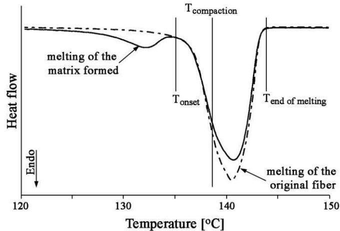
**Figure 4** DSC melting traces of a semicrystalline polymer fiber and its hot compacted version, schematically (based on [82])
