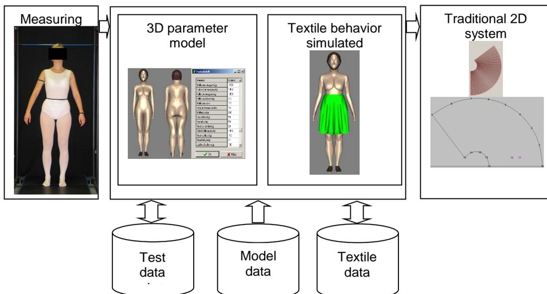
Figure 1 Structure of the System
