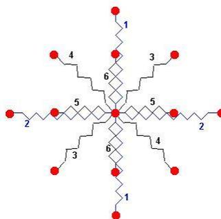
Figure 6 Springs and shock absorbers influencing a mass point.
