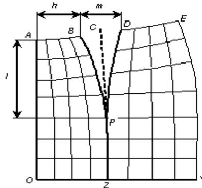
Figure 5 Position and sizes of contraction seams
