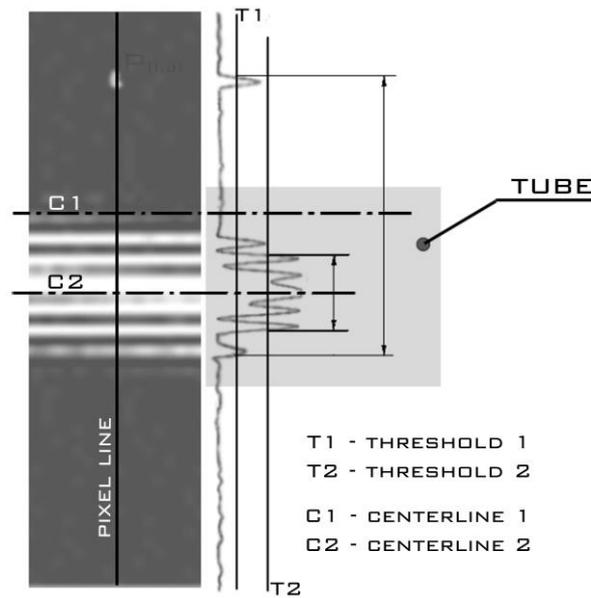
Figure 4 An example of pixel-graphic post processing of an image
