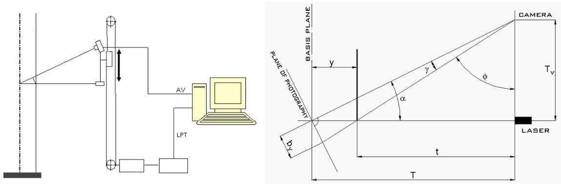
Figure 1 Operation principle of the 3D human body scanner
