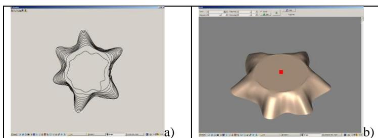
Figure 5: Captured contour after Fourier transformation (a) and recovered model (b)
