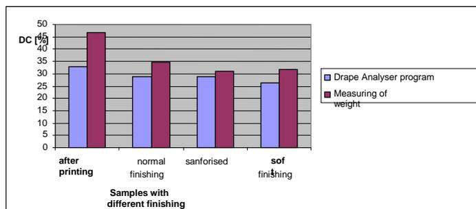
Figure 3. Drap coefficient of finished fabrics measured with different methods
