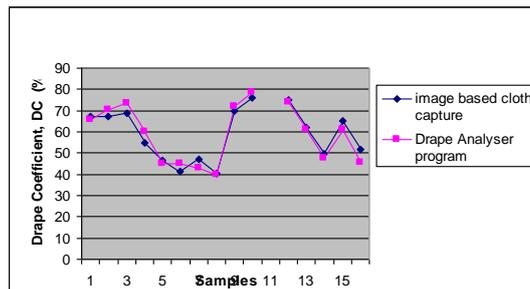
Figure 4.: Drap coefficient measured with image based capture and Drap Analyser program
