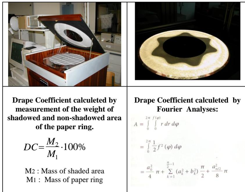
Figure 1: Different calculation methods of Drape Coefficient
