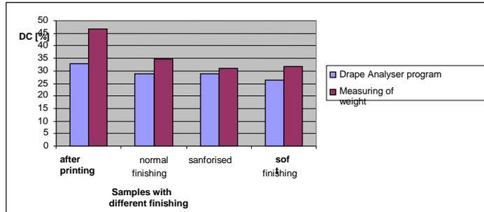
Figure 3. Drap coefficient of finished fabrics measured with different methods
