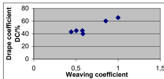
Figure 2: Influence of weaving coefficient of the fabrics with different pattern on drape coefficient DC
