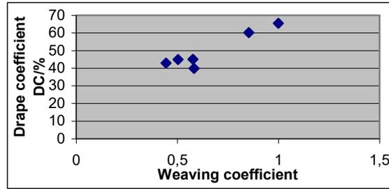
Figure 3 Influence of weaving coefficient of the fabrics with different pattern on drape coefficient DC
