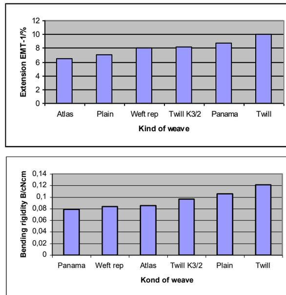
Figure 2 Influence of the fabric pattern on the mechanical properties of fabrics
