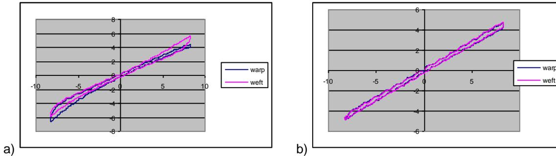
Figure 6 Shearing hysteresis of fabrics produced by different finishing a) before finishing; b) soft finishing
