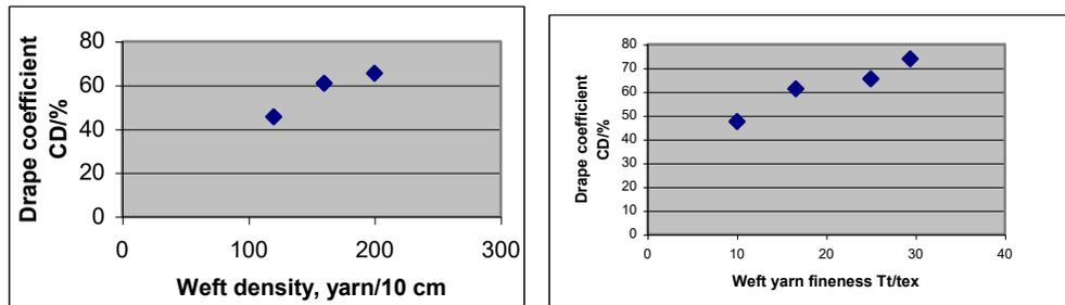
Figure 4 Drape coefficient CD of the fabrics with different weft yarn density fineness
