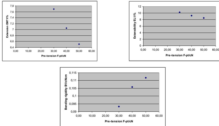
Figure 1 Influence of pre-tension of weft yarn on the mechanical properties of fabrics
