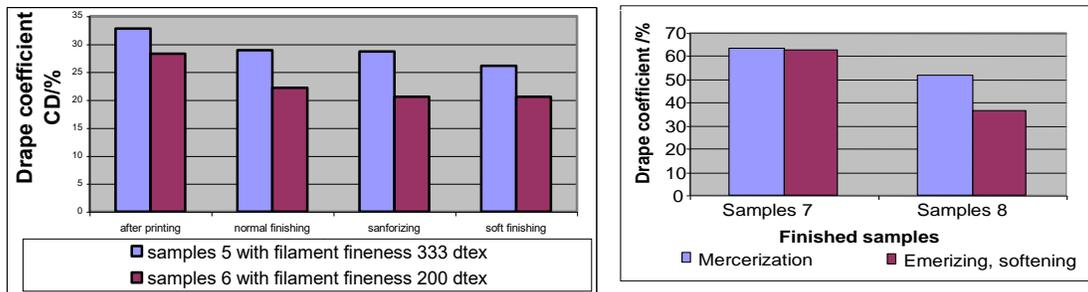
Figure 7 Drape coefficient of the fabrics produced by different finishing;
