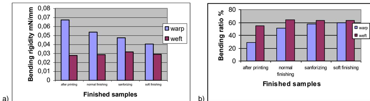
Figure 5 The effect of finishing on a) bending rigidity and b) bending ratio
