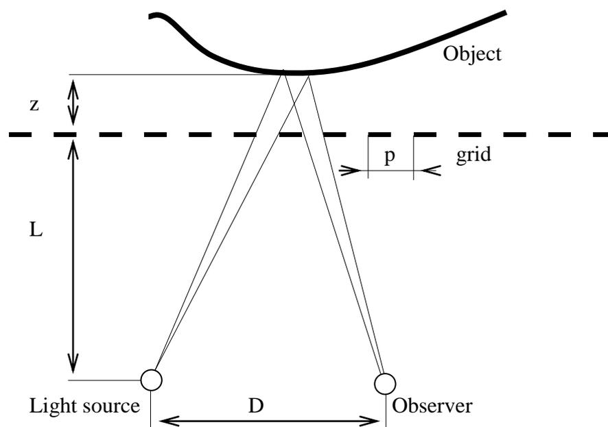
**Fig. 1.** The scheme of shadow moiré
