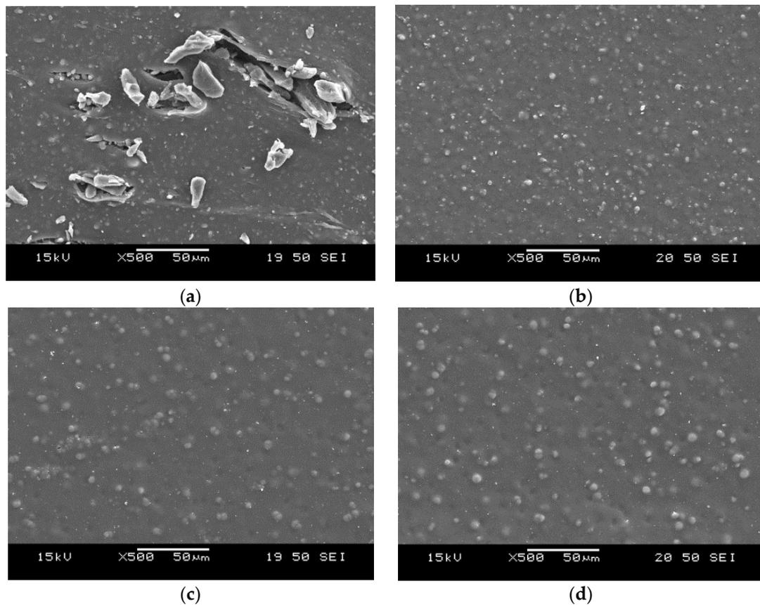
**Figure 7.** Cut surfaces of the SBR rubbers mixed at (a) 40 and (b) 140 and NBR rubbers mixed at (c) 40 and (d) 120 °C.
