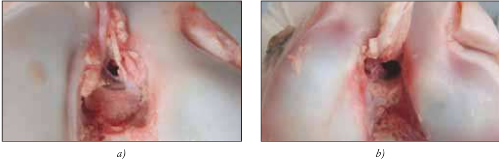
Figure 8. Femur head after pull out tests (a) tendon separated from the bone, (b) tendon broke. In both cases the screw remained behind in the bone tunnel with cancellous bone from the graft
