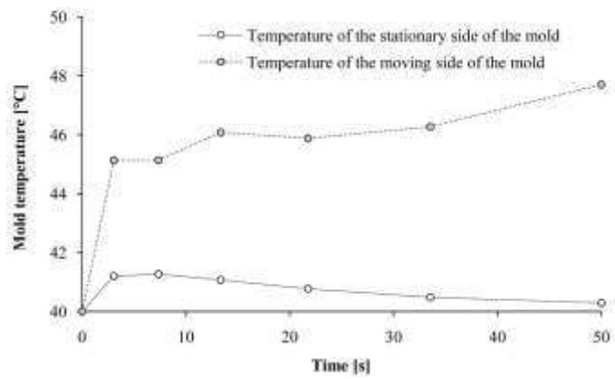
Fig.4. Mold temperature change at the corner as a function of time
