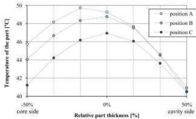
Fig.7. Temperature of the part 33 seconds after cavity filling
