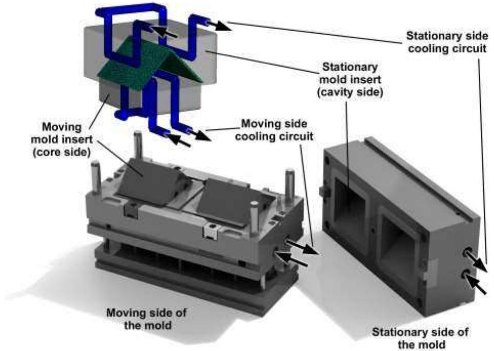
Fig.2. The injection mold with the model for the numerical simulation
