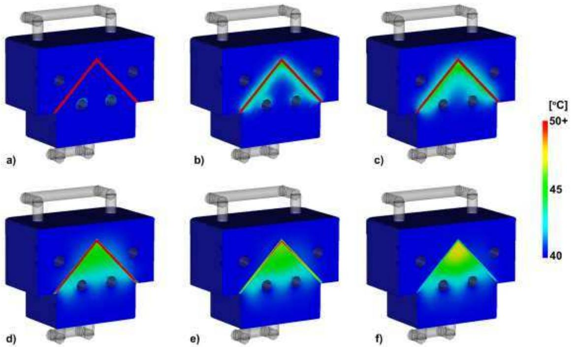
Fig.3. Temperature gradient through the injection molded part and the mold
