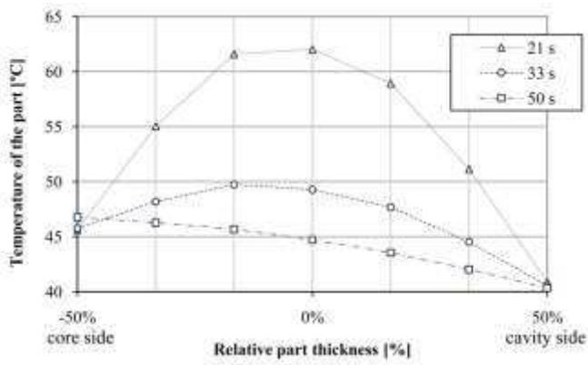
Fig.6. Temperature of the part at position A through the cross section
