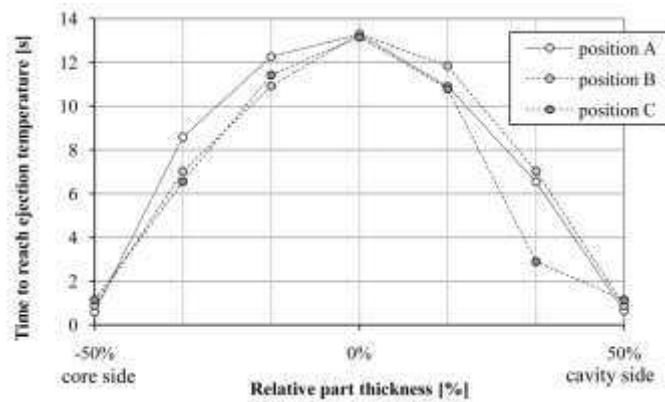
Fig.5. Time to reach ejection temperature at the corner along part thickness
