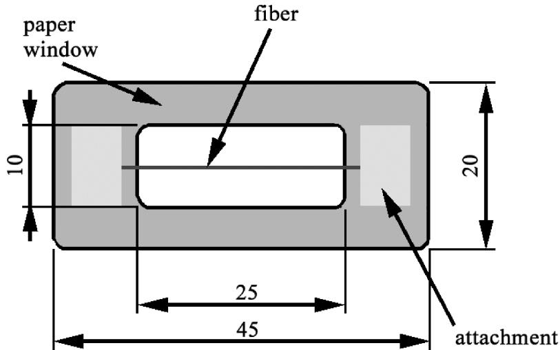
**FIGURE 3** Window frame used in the preparation for single fiber tests.
