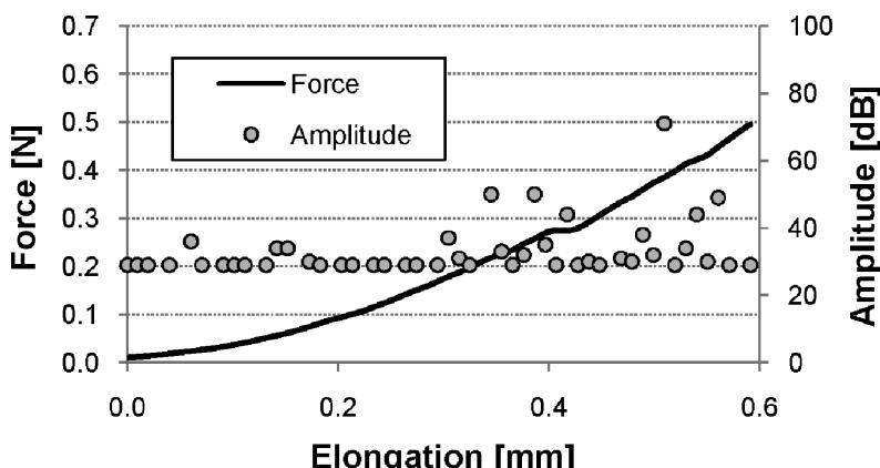
**FIGURE 10** Typical force and amplitude versus displacement curve for multifilament kenaf fiber.
