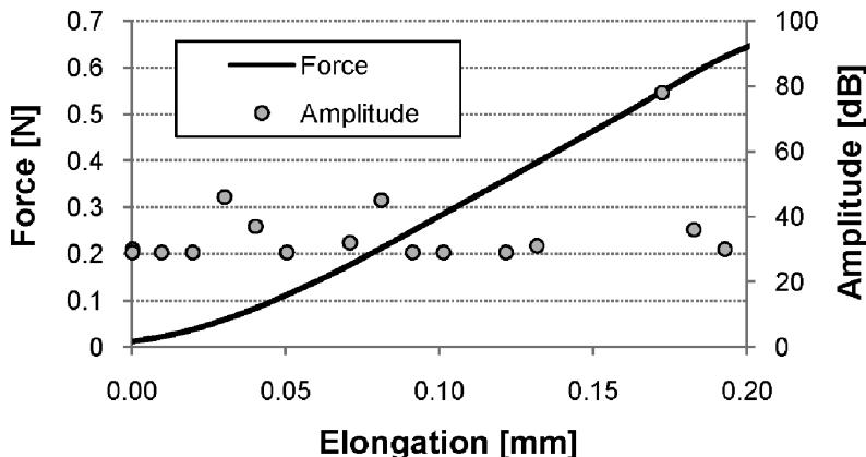
**FIGURE 9** Typical force and amplitude versus displacement curve for single kenaf fiber.
