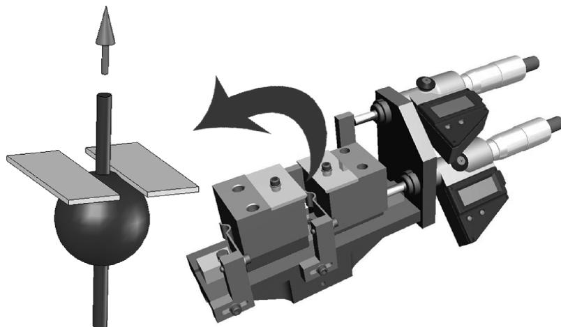
**FIGURE 1** Schematic diagram shows microdroplet test arrangement.
