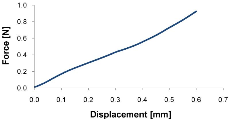
**FIGURE 8** Typical tensile curve obtained from single kenaf fiber test.
