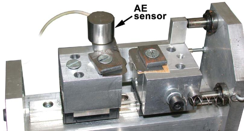
**FIGURE 4** Arrangement of the AE microphone.
