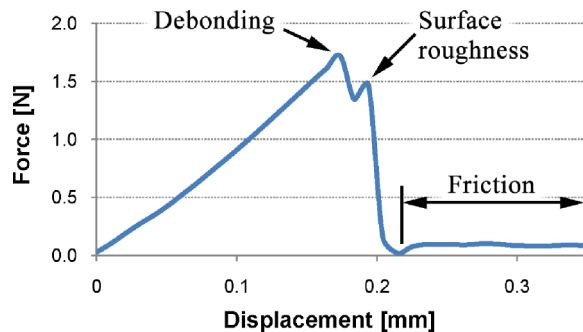
**FIGURE 6** Force–displacement curve for uneven surface of kenaf fiber.
