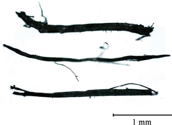
**FIGURE 7** Photomicrographs of kenaf fiber under optical microscope.
