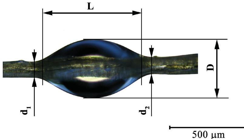
**FIGURE 2** Kenaf fibers with PLA matrix droplet.
