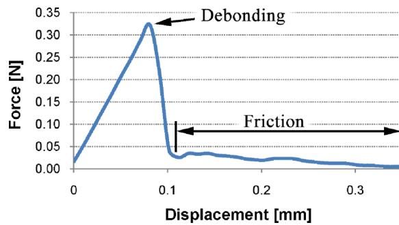
**FIGURE 5** Force–displacement curve obtained from microbond tests for single kenaf fiber.
