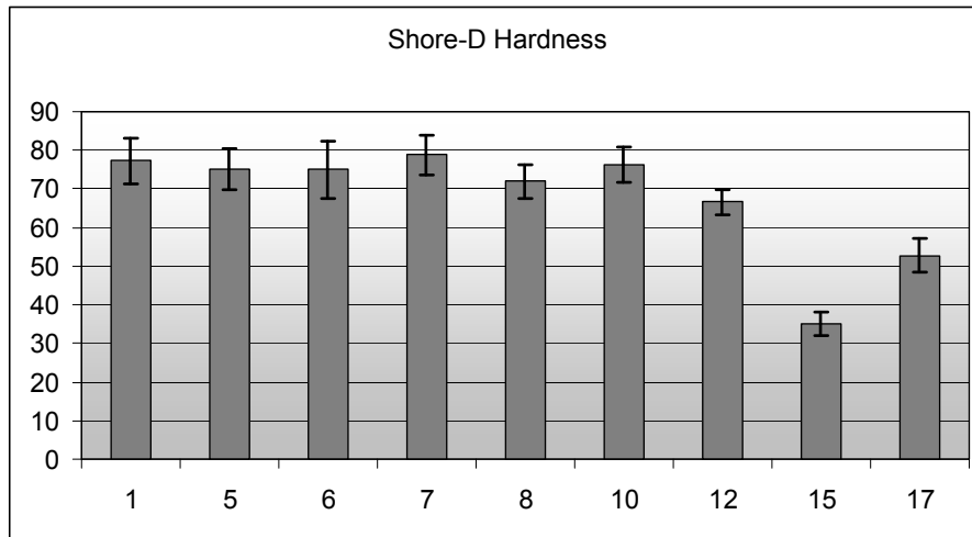
Fig. 2 Shore-D Hardness of examined epoxy resins
