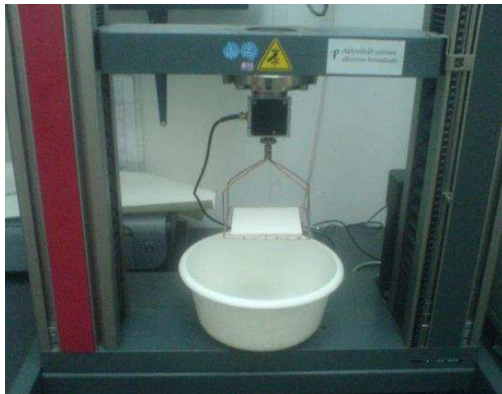
Fig. 3 Set up of the resin absorption measurement system
