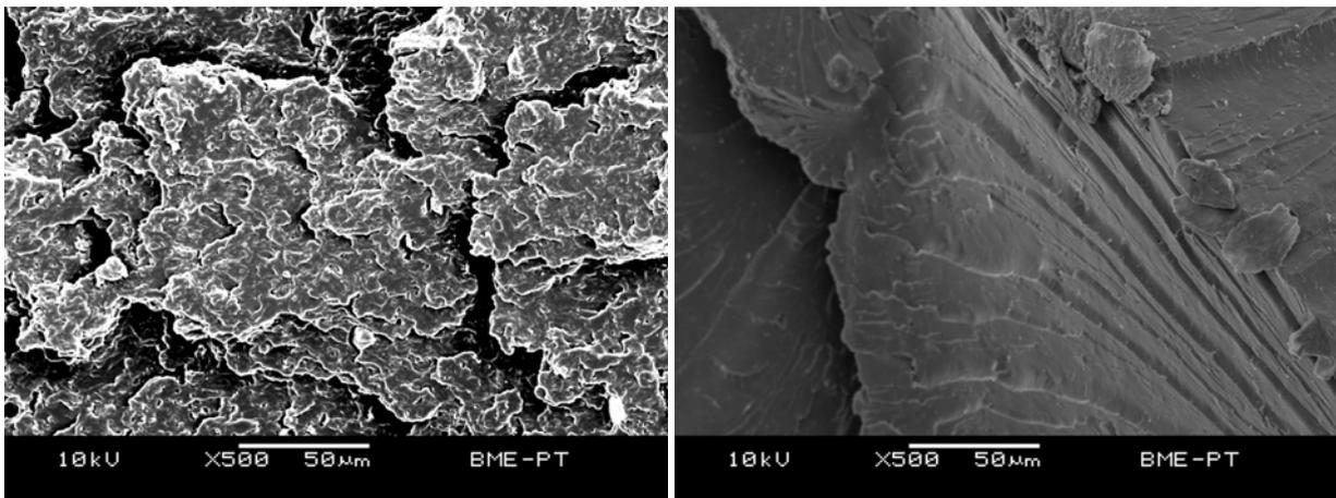
Figure 5. The fracture surface of the tensile specimens after 24 hours of ageing (left) and 168 hours of ageing (right)
