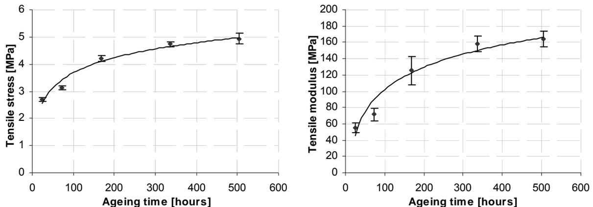
**Figure 1. The effect of ageing time on the tensile stress (left) and tensile modulus (right)**
