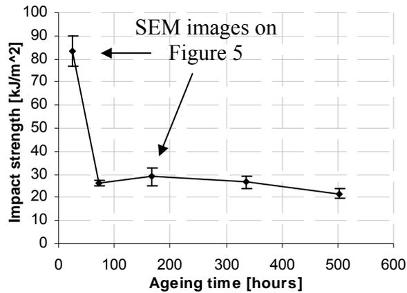
Figure 4. The effect of ageing time on the impact strength
