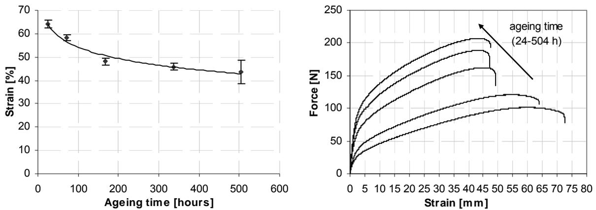
Figure 2. The effect of ageing time on the strain (left) and the changes in the tensile test diagrams (right)
