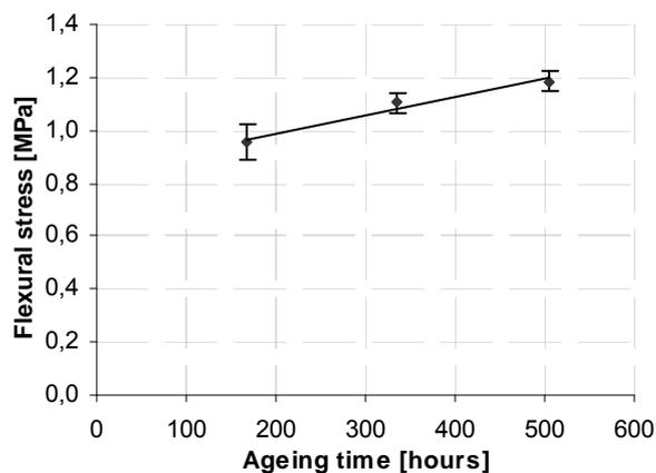
Figure 3. The effect of ageing time on the flexural stress
