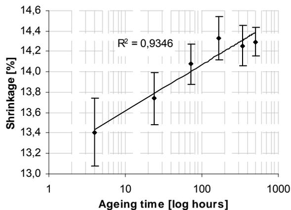
Figure 6. The effect of ageing time on the shrinkage
