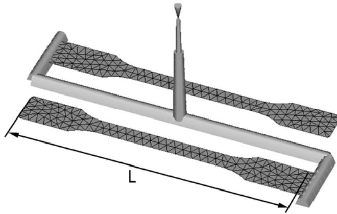
Fig.5. Model for tensile test specimen in MPI, used for shrinkage measurement (where L was the measured dimension)
