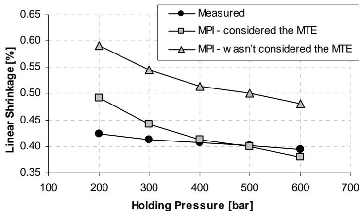
Fig.6. Shrinkage results where the packing pressure was varied between 20 MPa and 60 MPa (MTE is the Mold Thermal Expansion)
