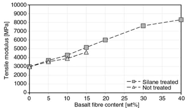
**Figure 3.** Tensile modulus of the basalt fibre reinforced PLA composites
