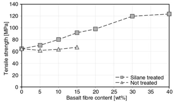
**Figure 2.** Tensile strength of the basalt fibre reinforced PLA composites
