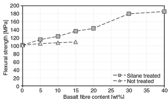
Figure 4. Flexural strength of the basalt fibre reinforced PLA composites
