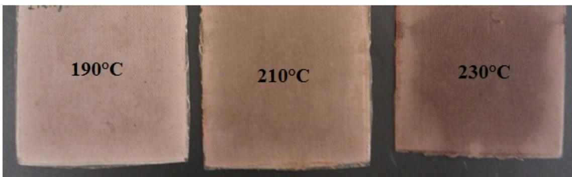
Fig. 3. Composites produced at 190, 210 and 230°C
