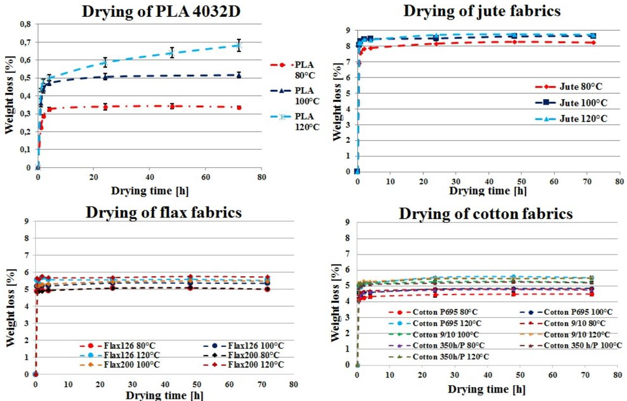
**Fig. 1. The drying characteristics of the materials**
