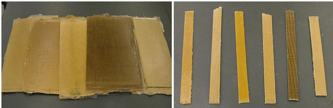
Figure 2. PLA/natural fibre composites made with compression moulding (left) and the test specimens (right)
