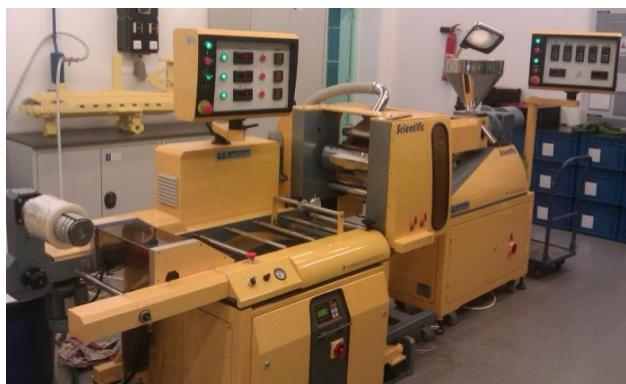
**Figure 1.** PLA film extrusion
