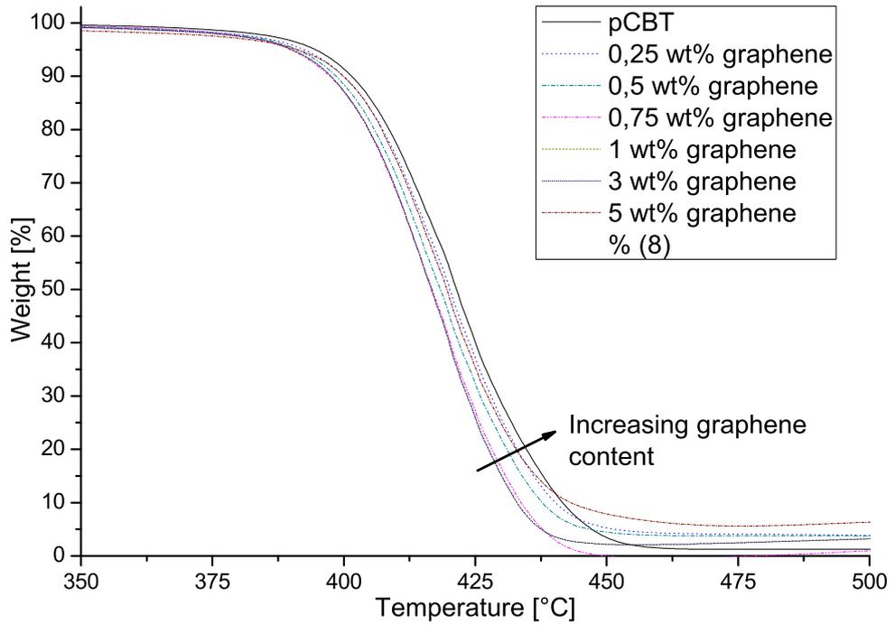
**Figure 5** Thermogravimetric curves of graphene-modified pCBT samples
