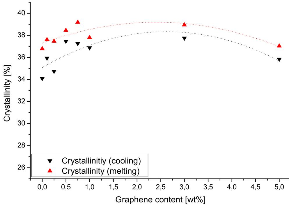
**Figure 2** Crystallinity in function of graphene content
