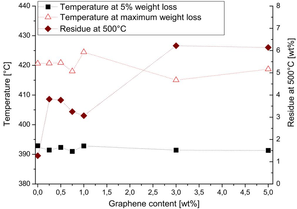
**Figure 6** Thermal decomposing properties of graphene-modified pCBT samples
