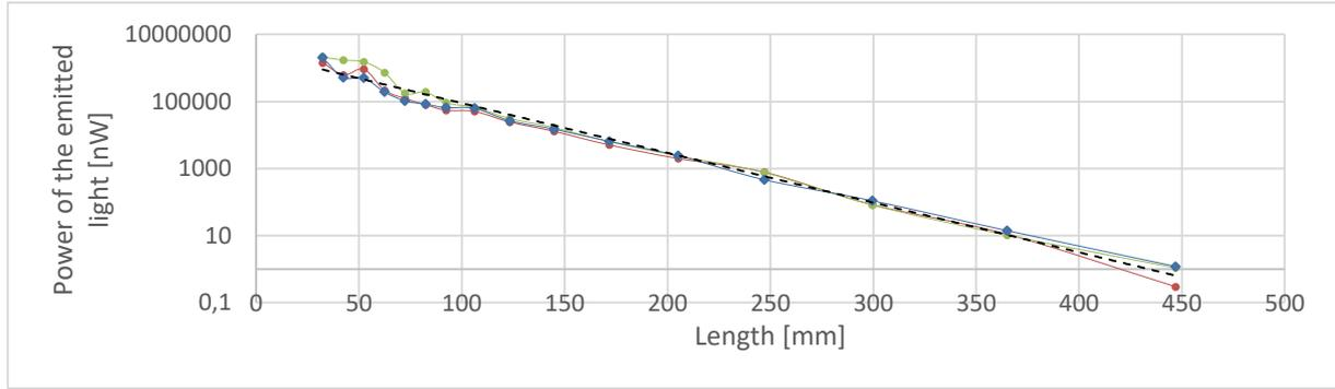
Figure 1: Light transmission graph of the fiber bundle in MR3012:MH3122 100:40 resin at different lengths
