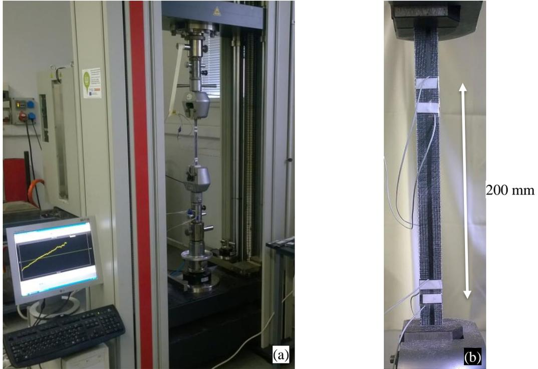
Figure 4: Measurement layout (a) and a close-up of the specimen (b)
