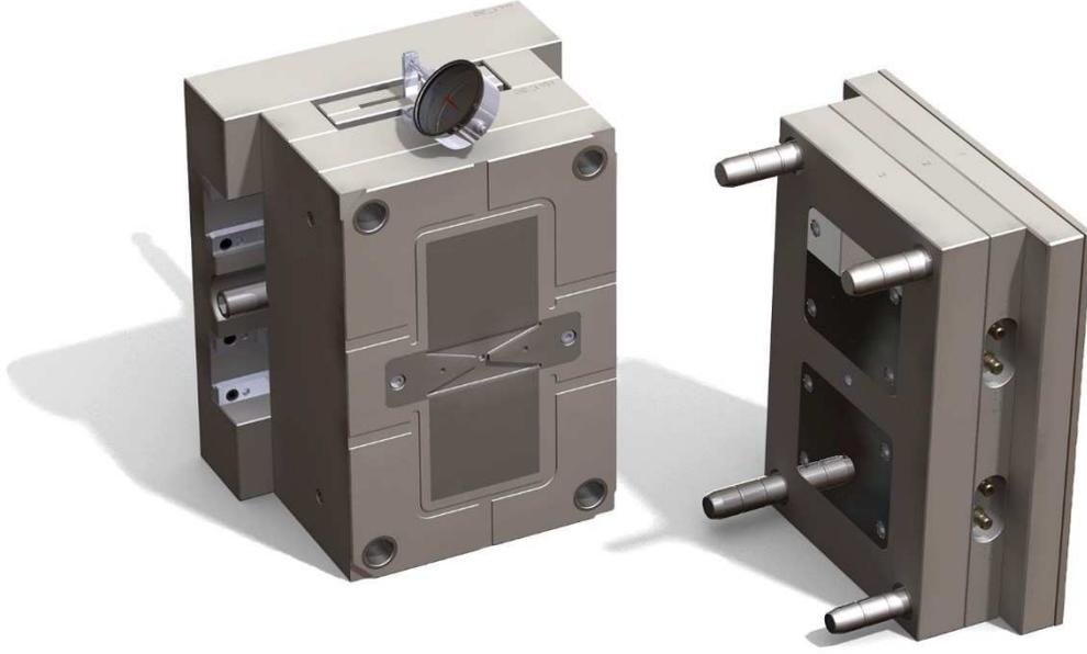
Figure 1. Test mold for color homogeneity evaluations
