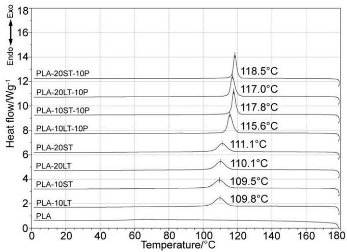
**Fig. 2** Cooling scan of compounds with small and large talc particle size measured at  $50^{\circ}\text{C min}^{-1}$
