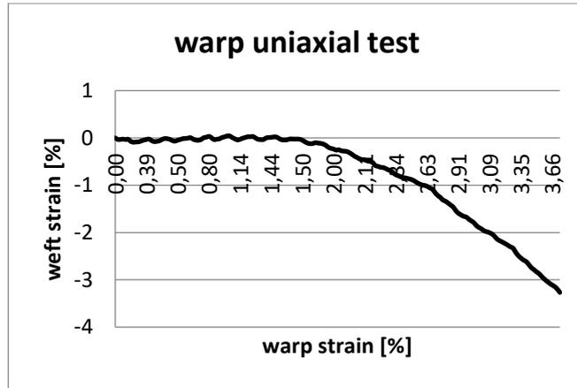
Figure 4. Transversal deformation, uniaxial test, warp loading.
