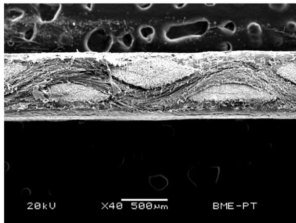
Figure 7. Microscopic photo of the section, the cut is parallel to the weft direction.
