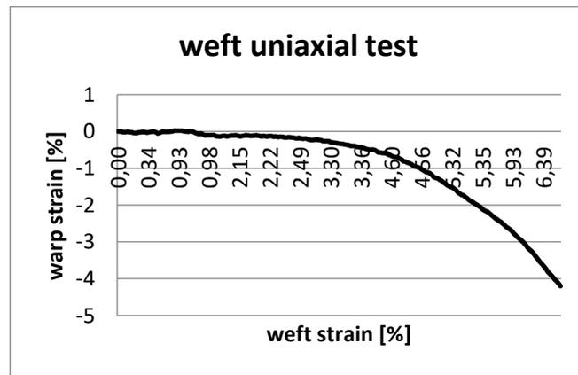
Figure 5. Transversal deformation, uniaxial test, weft loading.
