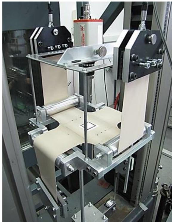
Figure 8. The bidirectional testing equipment.
