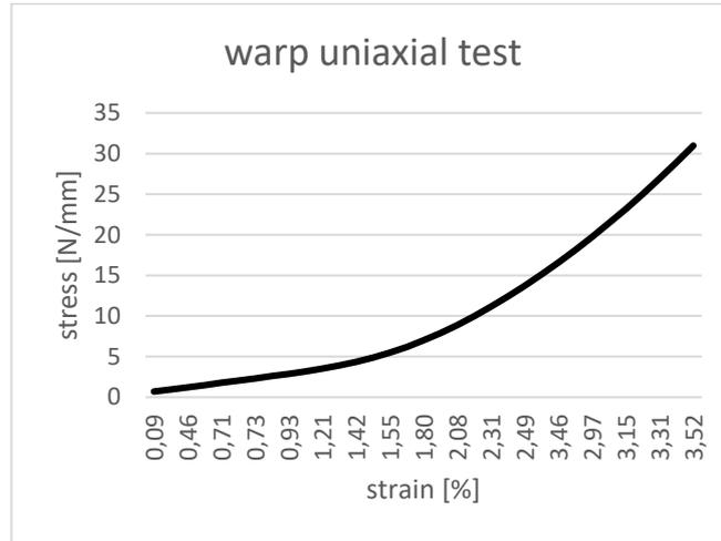
Figure 1. Measured stress, a typical stress-strain curve of a uniaxial tensile test in the warp direction.
