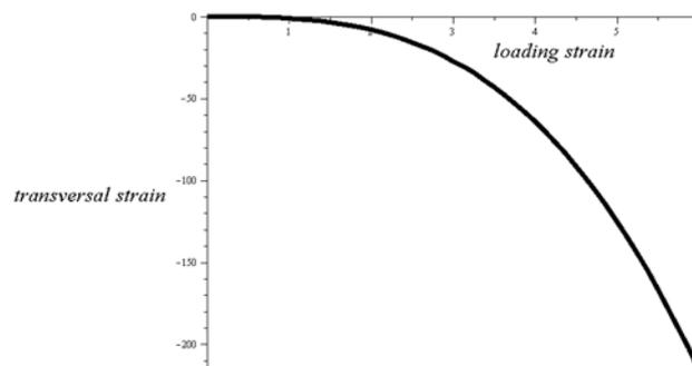
Figure 6. Calculated transversal deformation for uniaxial loading.
