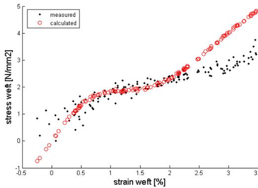
Figure 13. The uniaxial result of the parameter identification for the weft direction.
