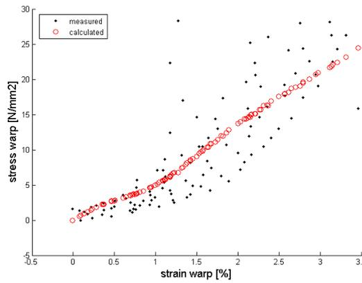
Figure 12. The uniaxial result of the parameter identification for the warp direction.
