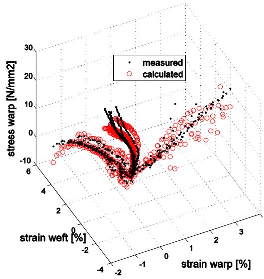
Figure 11. The general result of the parameter identification for the warp direction.
