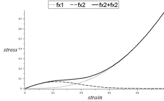
Figure 3. Calculated stress-strain diagram plotted by exponential functions.
