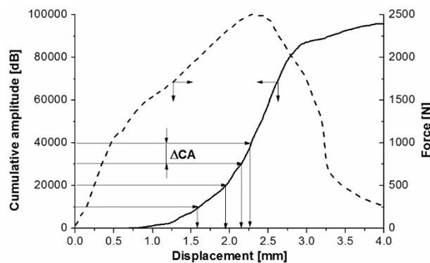
**Fig. 7.** Sectioning of the cumulative AE amplitude (CA) vs displacement curve of a thermoplastic starch composite containing 60 wt% flax in CP arrangement to get the same  $\Delta CA$  in each section. Note: this figure also contains the correspondent force-displacement curve. Reused by permission of Elsevier <sup>40</sup>
