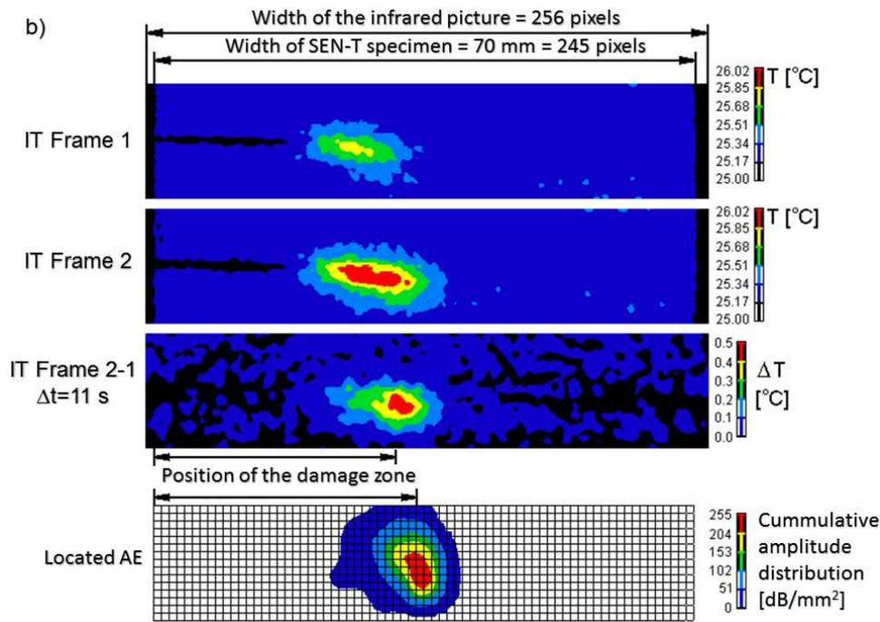
**Fig. 4.** Load-displacement curve registered on a SEN-T specimen of a thermoplastic starch composite containing 60 wt% flax in CP arrangement (a), and comparison of the damage zones derived from IT and AE measurements (b).<sup>40</sup> Notes: the temperature rise between IT frames 2 and 1 is calculated by considering the corresponding pixels. The AE damage zone covers 90 percentage surface related cumulative AE amplitudes. Reused by permission of
