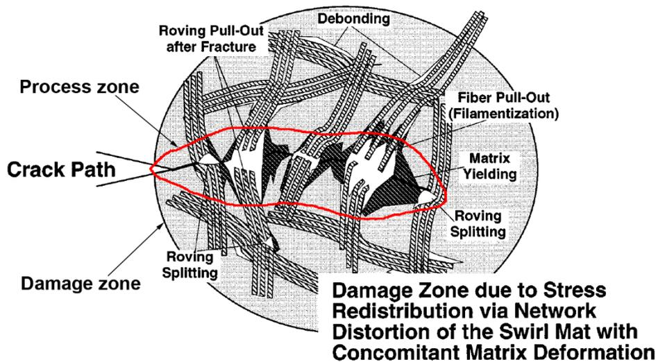
**Fig. 5.** Damage and process zones in glass mat reinforced thermoplastic composites (GMT) schematically<sup>41</sup>. Note: process zone is marked by red line. Reused by permission of Wiley<sup>41</sup>
