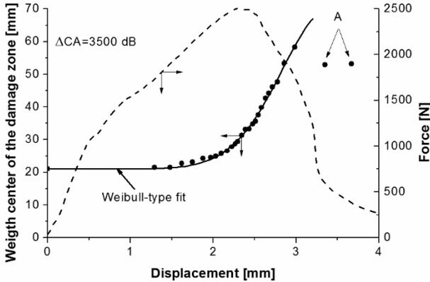
**Fig. 8.** Calculated crack growth in a SEN-T specimen of thermoplastic starch containing 60 wt% quasi unidirectional flax fiber in CP lay-up. Reused by permission of Elsevier <sup>40</sup>
