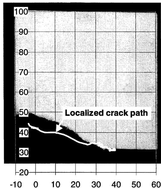
**Fig. 11.** Comparison of the real fracture path with that of the computed one through location of AE events. Notes: fracture path was computed by considering the advancing the center of gravity of the cumulative energy of AE. Material is a partly consolidated GMT-PP. Deviation between the localized and real fracture planes is due to pull-out events of long discontinuous GF. Scale is in millimeter. Reused by permission of Wiley-VCH <sup>34</sup>
