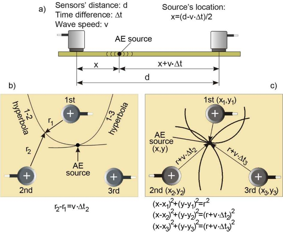
**Fig. 3.** Linear source location by two (a) and planar source location by three (b and c) sensors. Note: this figure also shows how the source is estimated by the interception of hyperbolae (b) and circles (c), respectively.
