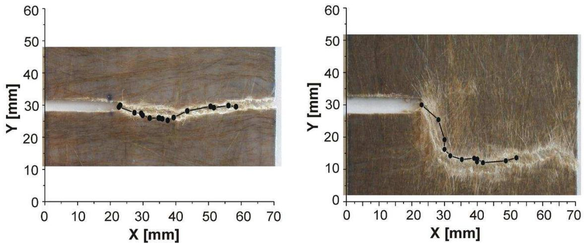
**Fig. 10.** Comparison of the real fracture path with that of the computed one through location of AE events. Notes: points along the continuous lines represent the movement of the center of gravity of the cumulative amplitudes of AE. Material is a thermoplastic starch with continuous flax fibers in CP lay-up
