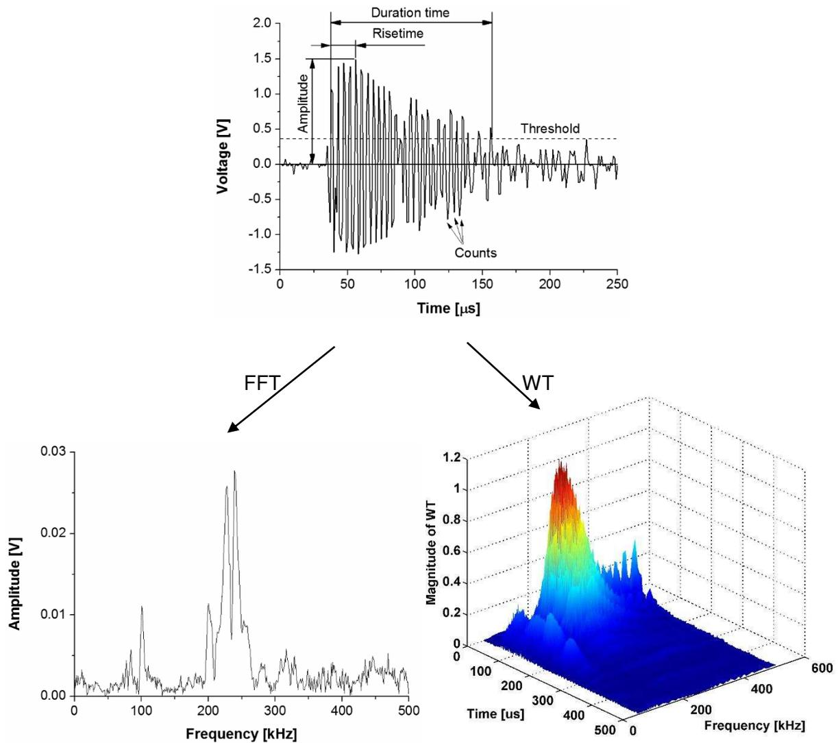
**Fig. 1.** Characteristics of a recorded burst-type AE event. This figure also shows the frequency- and time-frequency analyses of this burst AE event, captured after surpassing a preset threshold value. Frequency- and time/frequency-analyses were achieved by fast Fourier transform (FFT) and wavelet transformation (WT) techniques, respectively.
