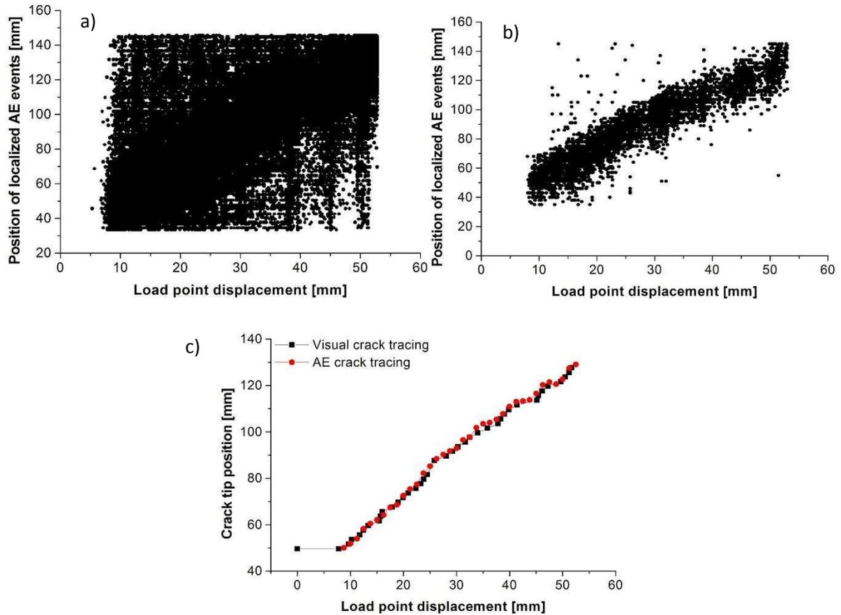
**Fig. 6.** The localized AE events before (a) and after filtering (b) of a hybrid composite DCB specimen with 0.1 wt% MWCNT. The crack traced by AE and visual inspection is displayed in (c). Reused by permission of BME-PT <sup>45</sup>
